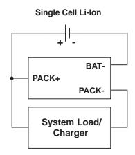
Figure 8. bq27x10EVM Circuit Module Connection to Cells and System Load/Charger
