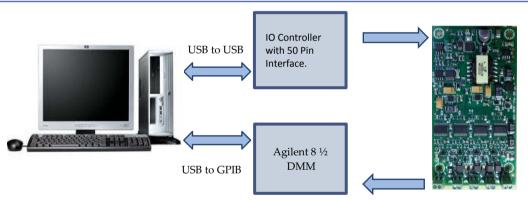
Note : For Voltage output the Load Resistance is >10k $\Omega$  and For current output the load resistance is 250ohms. **Figure 3 Functional Test Setup**
