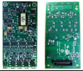
16-Bit Analog Output Module Reference Design for Programmable Logic Controllers (PLCs)
