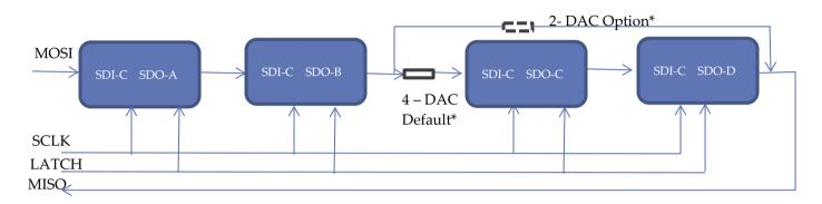
\*ONLY one of these two jumpers MUST be placed at any time. Refer the Schematic and BOM for the implementation.
