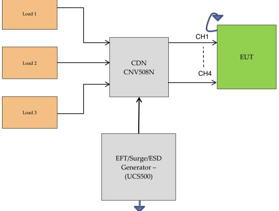
EUT operation monitored after the test. All the eight channels were monitored after the test by the Microcontroller (on IO Controller) and compared with a Set Value (equivalent of the external constant voltage or current source). The Error should be within accuracy as mentioned in Section 6.3.1. Method of monitoring:
