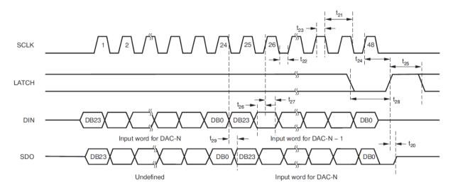
The SDO Pin is used to daisy chain the four devices together. As in a SPI, the rising edge of SCLK that clocks in the MSB of the input frame marks the beginning of WRITE cycle. When the serial transfer to all the devices is complete, LATCH is made HIGH. This action transfers the data from SPI shift registers to the device internal registers of the respective DAC. The number of clocks in each frame depends on the number of devices. Each frame is of Nx24 clocks.
