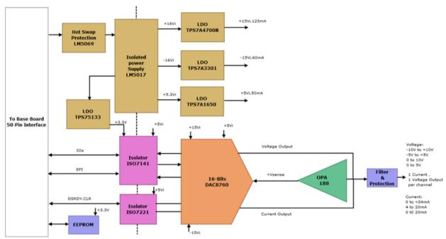
Figure 1 Block Level Design
