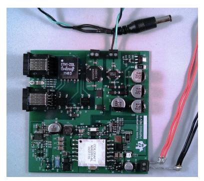
Figure 9. PMP6659 AC-Adapter Input Setup
