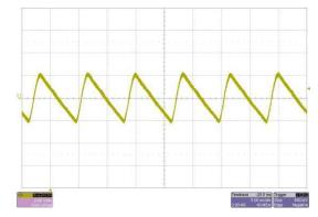
Figure 17. Input Ripple Across C27 with a 24-V AC Input, 2 V/div, 5 ms/div
