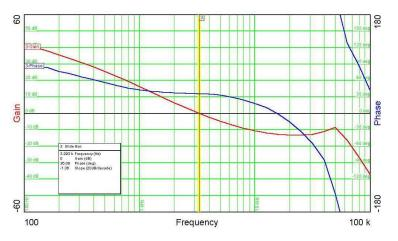
Figure 25. Loop Gain and Phase Margin at 12 V
