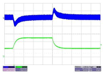
Figure 18. Load Step, 48 V<sub>1</sub> at J2 100 mV/div, 500 µs/div
