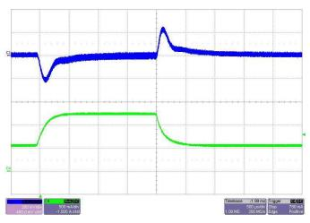
Figure 19. Load Step, 12 V<sub>1</sub> at J3 200 mV/div, 1 ms/div
