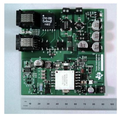
Figure 3. The PMP6659 Board (Revision B)
