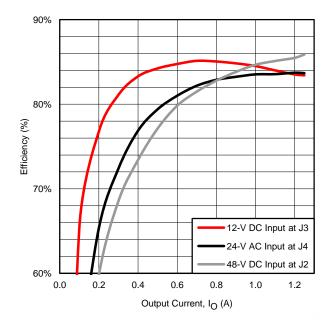
Figure 12. Efficiency of the PMP6659 Across a Wide Input Range
