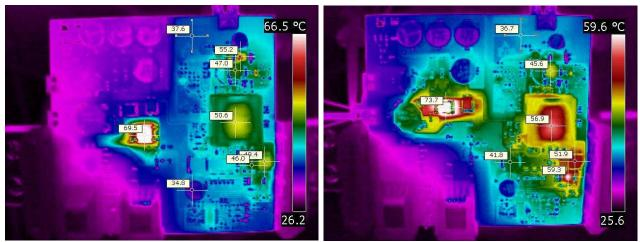
Figure 26. 48-V Input and 1.25-A Load
