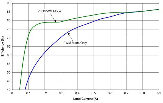
Figure 2. TPS23751 and TPS23752 Light Load Efficiency Versus Mode
