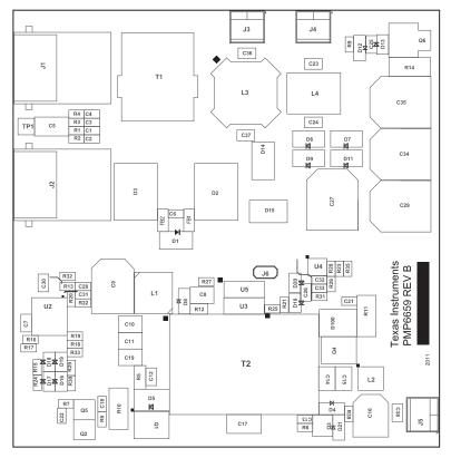
Figure 31. PMP6659 Assembly Drawing
