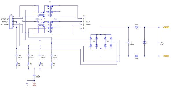
Figure 10. PMP6659 PoE Input Schematic
