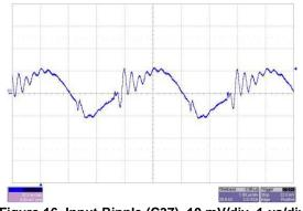
Figure 16. Input Ripple (C37), 10 mV/div, 1  $\mu s/div$
