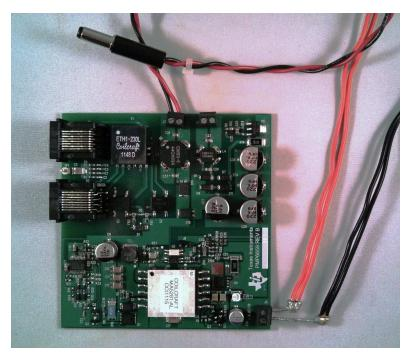
Figure 7. PMP6659 DC-Adaptor Input Setup
