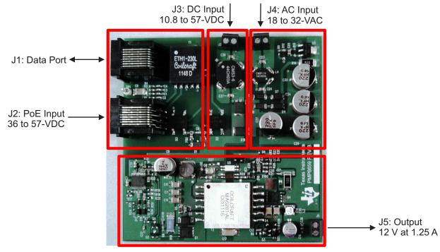
Figure 5. PMP6659 Inputs and Outputs
