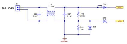
Figure 6. PMP6659 DC-Adaptor Input Schematic
