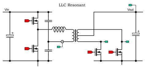
Figure 1. TMDSHVRESLLCKIT Circuit Diagram
