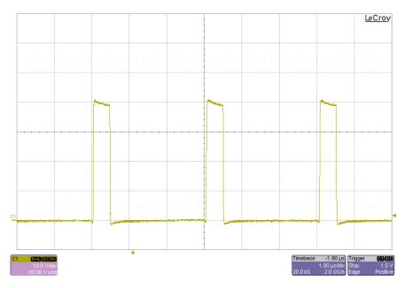
The following figure shows the switch node at 40Vin and 2.5 amp out.
