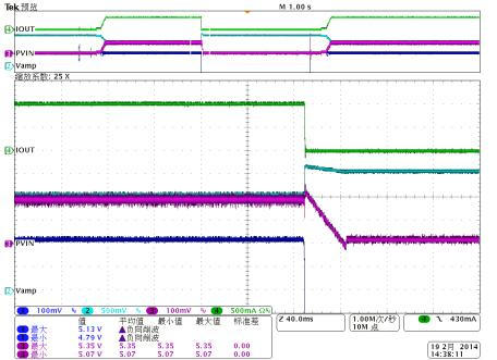
Figure 17 Circuit response with tablet attach (plug-in) event (DCP\_Auto Mode change)
