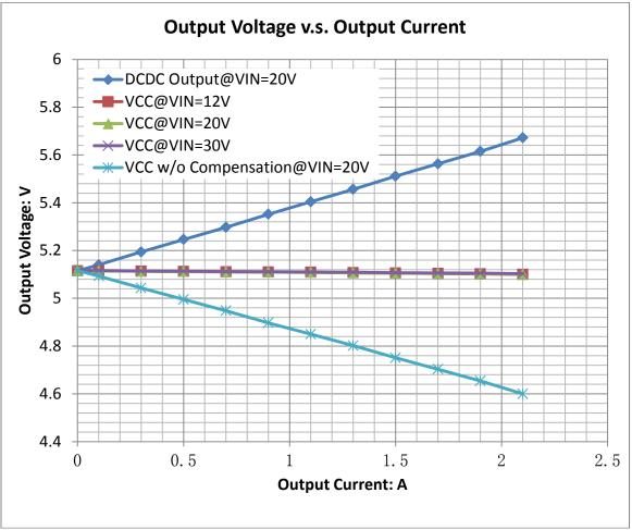
Figure 2 Output compensation versus load current
