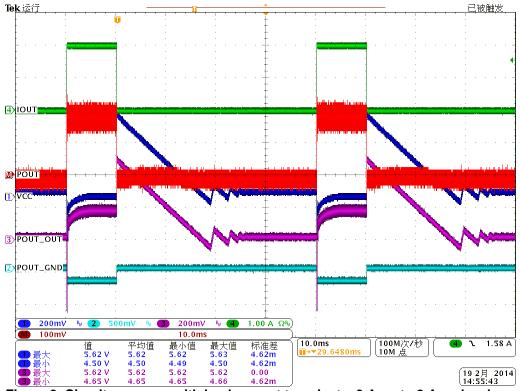
Figure 9 Circuit response with load current transients, 0 Amp to 2 Amp levels
