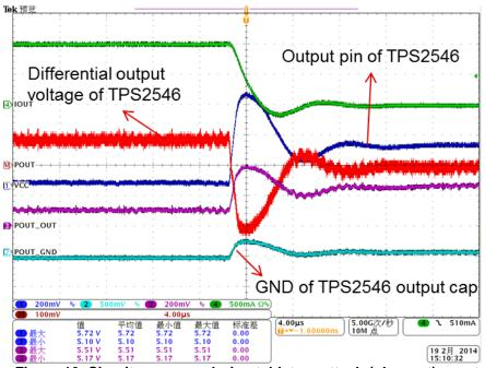
Figure 19 Circuit response during tablet un-attach (plug-out) event - tablet unplugs from device cable
