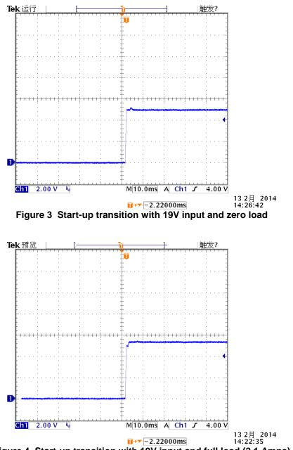
Figure 4 Start-up transition with 19V input and full load (2.1 Amps)
