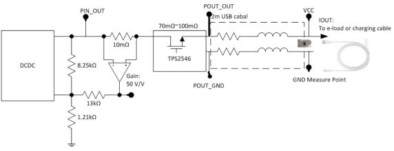
Figure 8 Dynamic load transient measurement scheme
