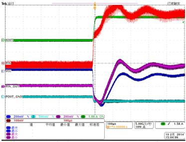
Figure 11 Detail of 0 Amp to 2 Amp load transient
