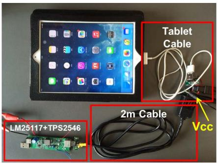
Figure 15 USB device charging test set-up
