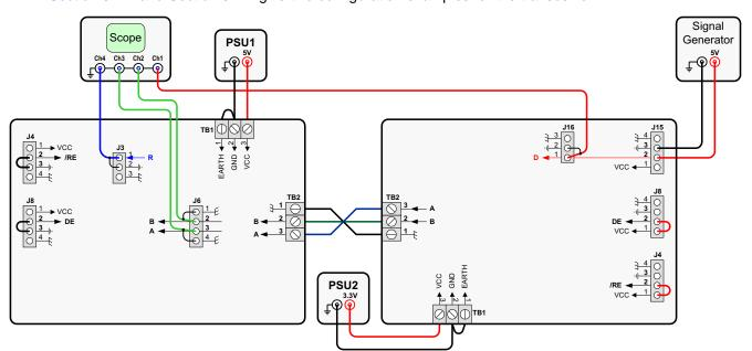
Figure 16. RS-485 BoosterPack Setup for Standard Measurement Configuration
