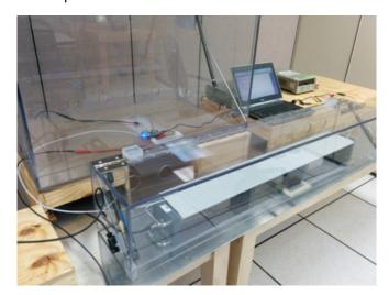
Figure 28. IEC61000-4-4 EFT Test Setup
