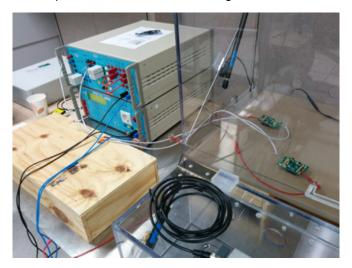
Figure 29. IEC61000-4-5 Surge Test Setup
