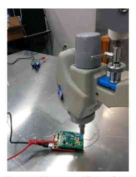
Figure 30. IEC61000-4-2 ESD Test Setup
