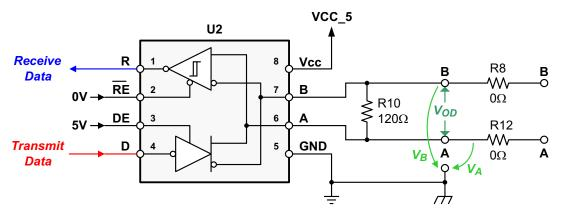
Figure 17. Transceiver Configuration for Normal Operation
