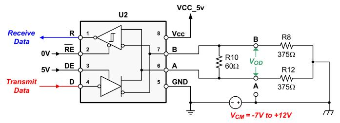
Figure 19. Configuration for Maximum Loading
