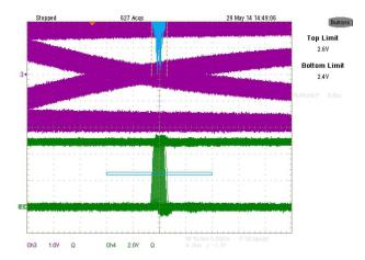
Figure 24. Output Jitter at 3-Mbps Data Rate Over 1024 Feet of Cable
