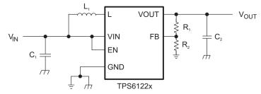
Figure 9. Application Circuit For Adjustable Output Voltage Option
