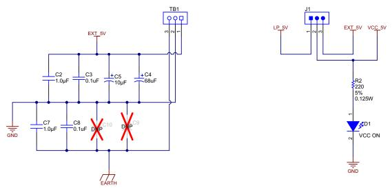
Figure 11. External Power Supply Implementation
