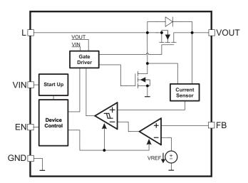
Figure 4. TPS61220 Functional Block Diagram
