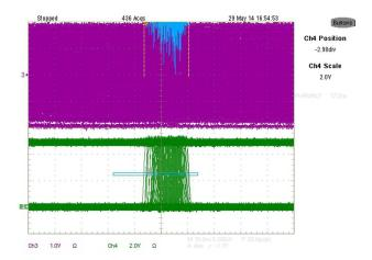
Figure 25. Output Jitter at 12.5-Mbps Data Rate Over 1024 Feet of Cable
