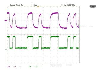
Figure 27. Level-Shifter Output at 1.25-Mbps
