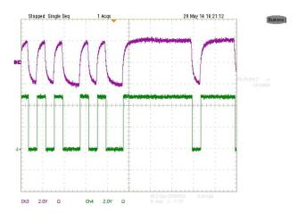
Figure 26. Transceiver Output at 1.25-Mbps
