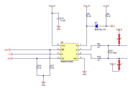
Figure 8. Transceiver Final Design
