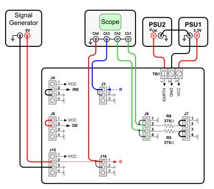
Figure 20. RS-485 BoosterPack Setup for Maximum Loading
