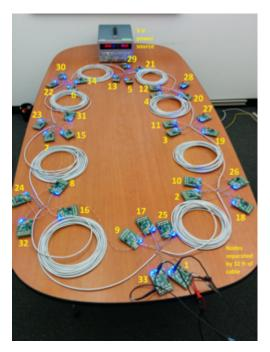
Figure 21. RS-485 Test Setup
