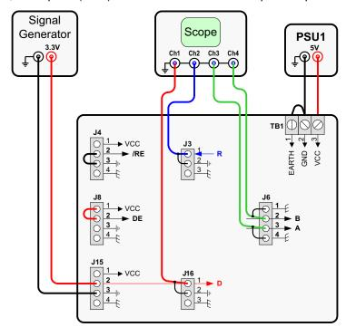
Figure 18. RS-485 BoosterPack Setup for Normal Transceiver Operation
