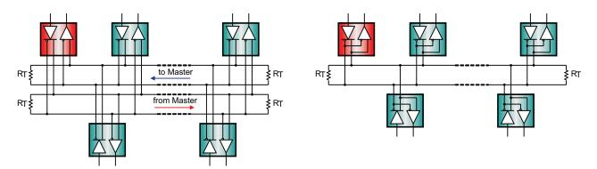
Figure 7. Full-duplex and Half-duplex Bus Structures in RS-485
