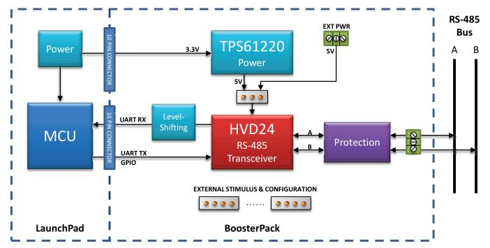
Figure 2. BoosterPack Block Diagram
