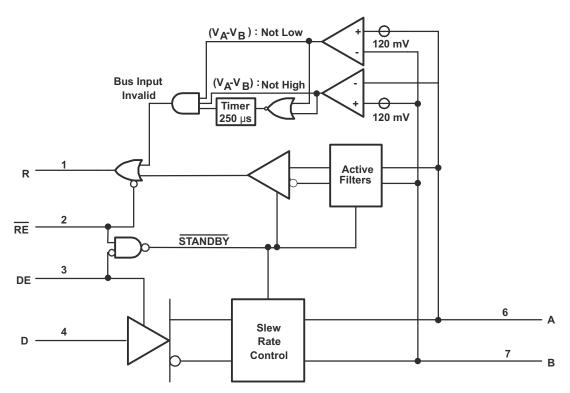
Figure 3. SN65HVD24 Functional Block Diagram
