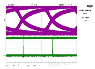
Figure 23. Eye Diagram at 3-Mbps Data Rate Over 1024 Feet of Cable
