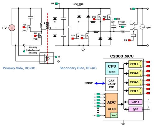
Figure 1. Solar Micro Inverter Kit Power Stage Diagram
