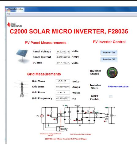
Figure 5. Solar Micro Inverter Release GUI
