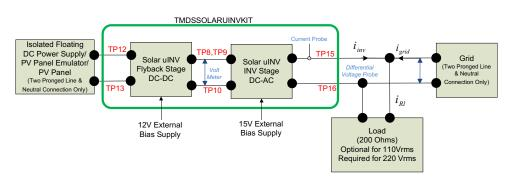
Figure 3. Solar Micro Inverter Kit Demo Setup
