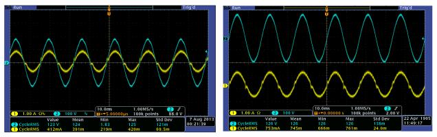
Figure 6. Output Volt and Current at 110-V, 60-Hz Grid Volt. Input 35-V DC, Input Current 2.25-A DC, Ch2 Vout, Ch4 Iout Figure 7. Output Volt and Current at 126-V<sub>RMS</sub>, 60-Hz Grid Volt. Input 44-V DC, Input Current 2.0-A DC, Ch2 Vout, Ch4 Iout
