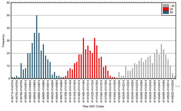
Figure 59. Noise Histogram of RTD Channel
