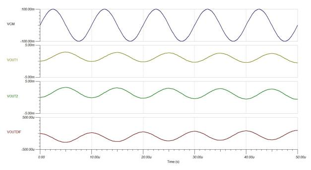
Figure 30. Mismatched Common-Mode Capacitors
