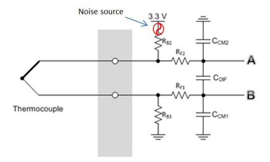
Figure 41. Biasing Resistors Noise Model
