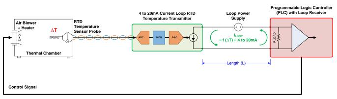
Figure 18. Typical Block Diagram of a Current Loop System
