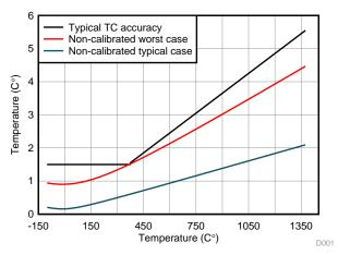
Figure 44. Calculated Error in °C as a Function of the Measured Temperature
