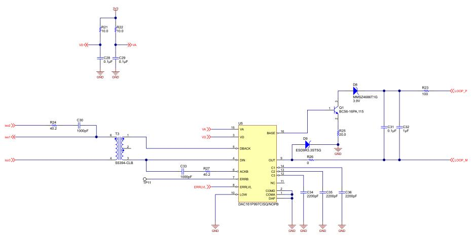
Figure 76. Schematic - Loop Current - DAC
