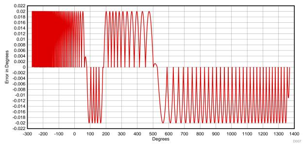
Figure 50. Examples of the Error Intruded by the Software by Using Different Look Up Tables
