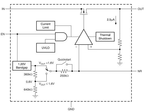
Figure 24. TPS71733 – Functional Block Diagram
