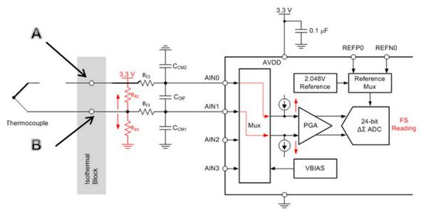
Figure 43. Improved Biasing Circuit
