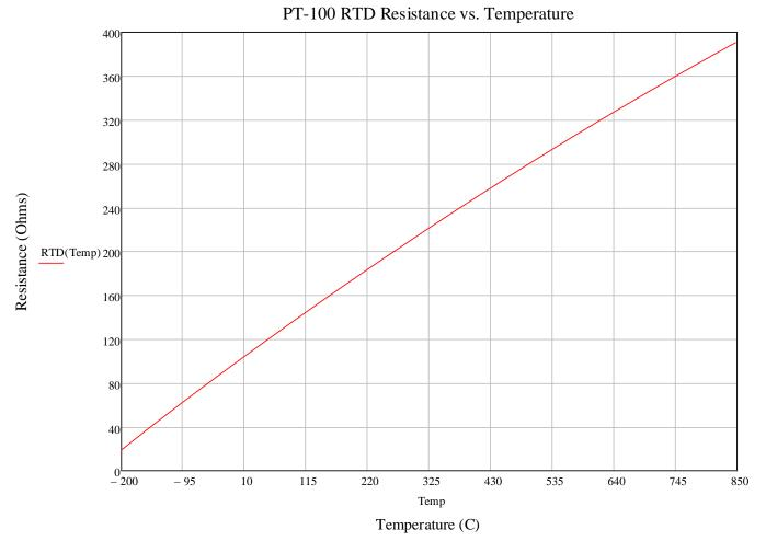
Figure 13. RTD Resistance and Linear Fit Line Versus Temperature
