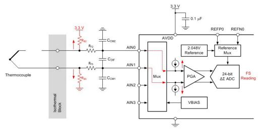
Figure 39. Biasing Resistors RB1 and RB2
