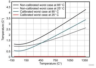
Figure 49. Worst Case Calibrated and Non-Calibrated Total Front End Error (at 25°C and 85°C)
