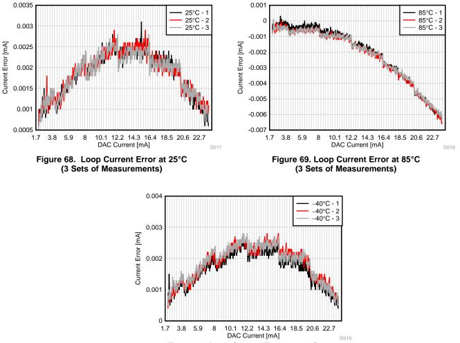
Figure 70. Loop Current Error at -40°C (3 Sets of Measurements)
