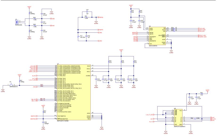
Figure 77. Schematic - Analog Front-End, MCU, and Isolated Data
