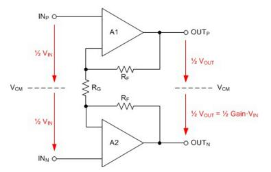
Figure 40. Common-Mode Voltage Limitation in the ADS1220
