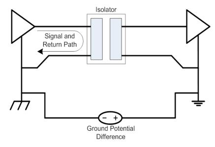
Figure 16. Galvanic Isolation Breaks Ground Loops
