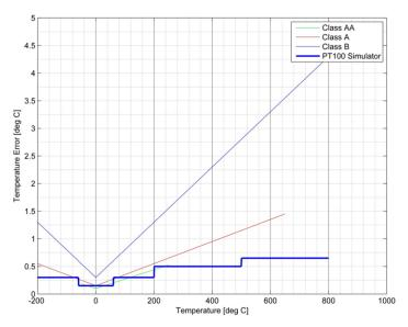
Figure 58. Temperature Error vs Temperature of PT100 Sensors (Class AA, A, B) and PT100 Simulator
