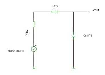
Figure 42. Simplified Circuit for R<sub>Bias</sub> Noise
