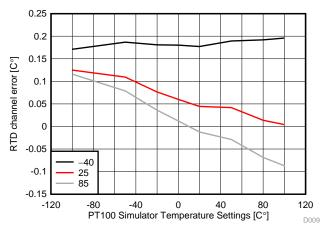
Figure 60. Temperature Error of the RTD Channel
