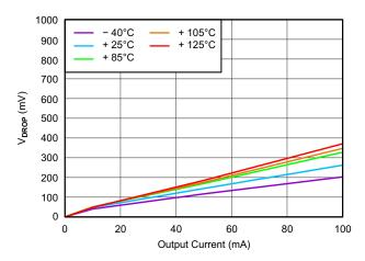
Figure 22. TPS7A1601 - Dropout Voltage vs. Output Current
