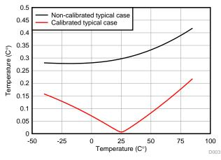
Figure 46. Typical Calibrated and Non-Calibrated Error of RTD
