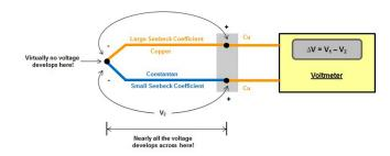
Figure 5. Thermocouple and Developed Voltage
