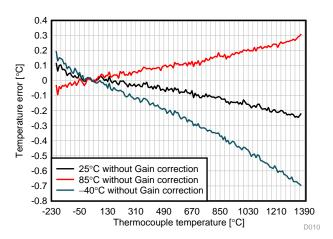
Figure 61. Temperature Error Without Gain Correction Over Temperature
