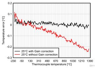
Figure 62. Temperature Error With and Without Gain Correction at 25°C
