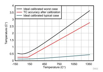
Figure 45. Calculated Error in °C as a Function of the Measured Temperature in a Calibrated System
