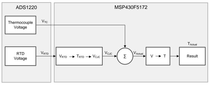
Figure 51. Software Flow Diagram for Thermocouple Linearization
