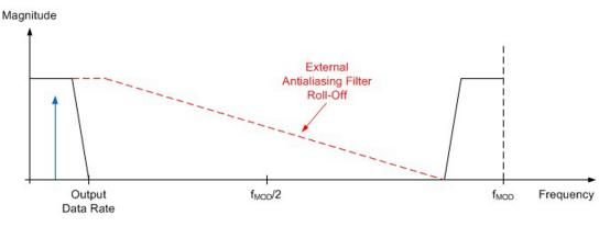
Figure 35. Antialiasing Filter
