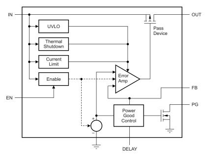
Figure 21. TPS7A1601 Block Diagram
