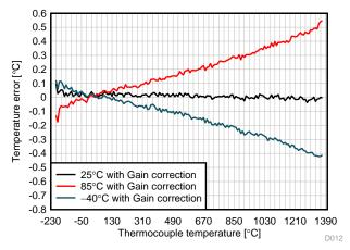
Figure 63. Temperature Error With Gain Correction Over Temperature
