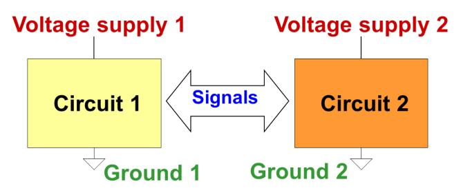
Figure 17. Definition of Galvanic Isolation
