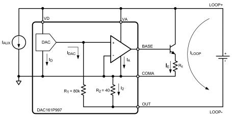
Figure 27. DAC161P997 Block Diagram
