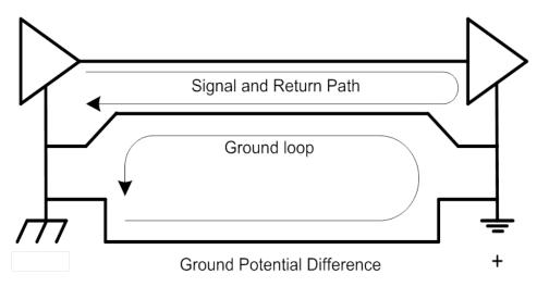
Figure 15. Ground Loops in Presence of Different Ground Potentials
