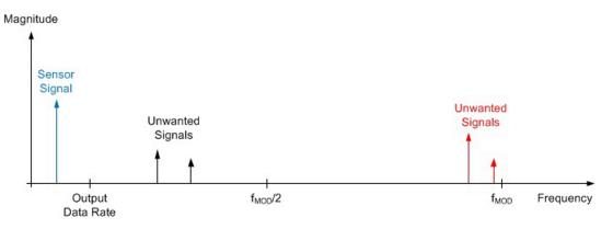
Figure 33. Unwanted Signal in the Frequency Domain
