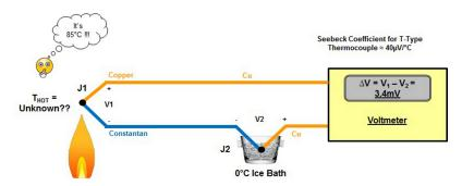
Figure 11. Measuring Absolute Temperature Using 0°C Ice Bath
