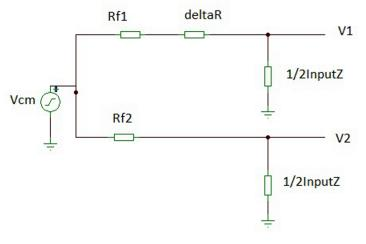
Figure 38. Simplified Circuit of R<sub>f1</sub> Mismatched
