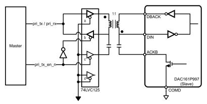
Figure 20. Isolate Signal Path Block Diagram (SWIF plus Transformer)
