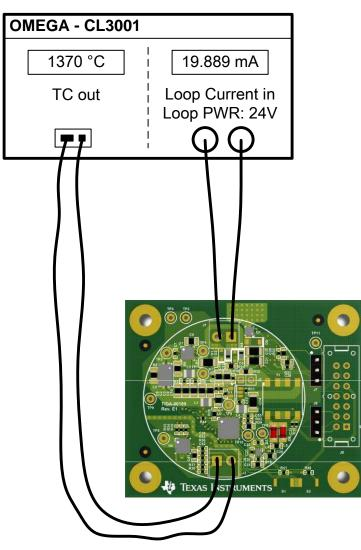
Figure 56. Basic Test Setup
