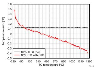
Figure 65. Temperature Error with Cold Junction Compensation, Measured Cold Junction (Set to 0°C) at 85°C Ambient Temperature
