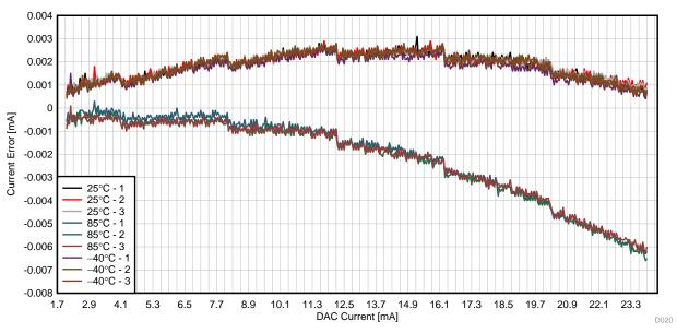
Figure 71. Loop Current Error Over Ambient Temperature
