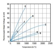
Figure 6. Thermocouple Output as Function of Temperature
