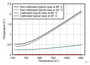
Figure 48. Typical Calibrated and Non-Calibrated Total Front End Error (at 25°C and 85°C)
