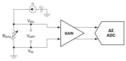
Figure 12. Simplified RTD Application Circuit
