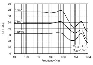
Figure 23. TPS71733 – PSRR vs. Frequency @ VIN – VOUT = 0.25V
