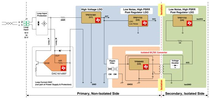
Figure 55. Block Diagram of Power Supply and Loop Input Protection
