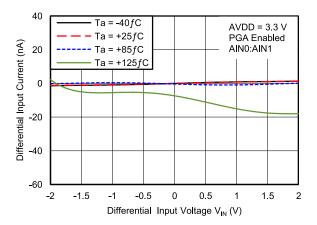
Figure 37. Differential Input Current vs Differential Input Voltage (PGA Enabled)
