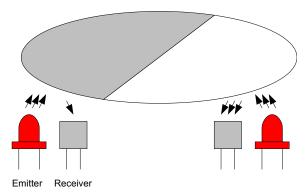
Figure 1. Optical Sensor using Coding Wheel for Rotation Detection
