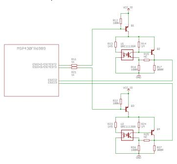
Figure 3. Connection Between Optical Sensors and the MSP430FR6989
