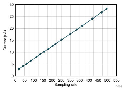
Figure 5. Sampling Rate versus Power Consumption
