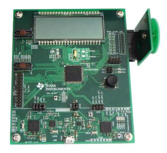
Figure 4. EVM430-FR6989 Main Board with Optical Sensor Board Attached
