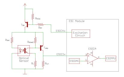
Figure 2. Optical Sensor with ESI
