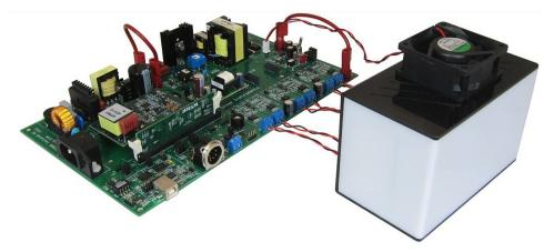
Figure 1. The AC LED Lighting and Communications Developer's Kit
