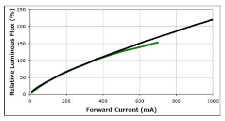
Figure 3. LED Current versus Luminous Flux
