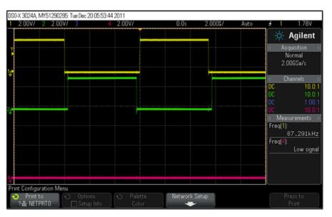
Figure 22. LLC PWM Waveforms at 85.7 kHz
