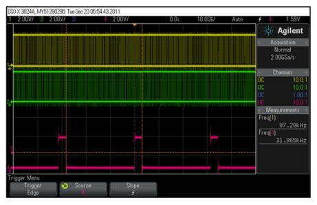
Figure 23. LED0 PWM Waveform at 10% Duty Cycle
