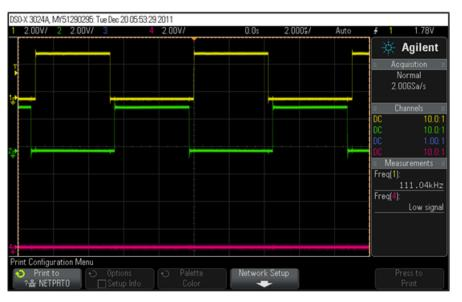
Figure 21. LLC PWM Waveform at 110 kHz
