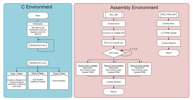
Figure 27. Incremental Build 2 Software Flowchart
