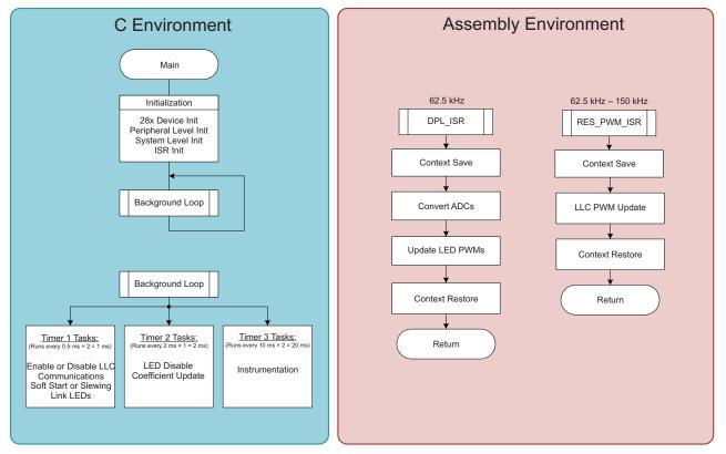
Figure 19. Incremental Build 1 Software Flowchart
