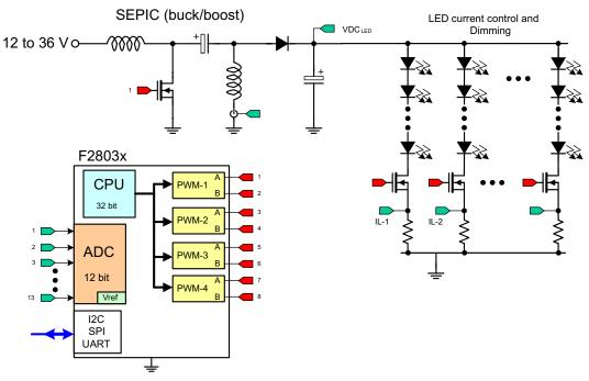
Figure 6. PWM Dimmed Strings with a Common Supply
