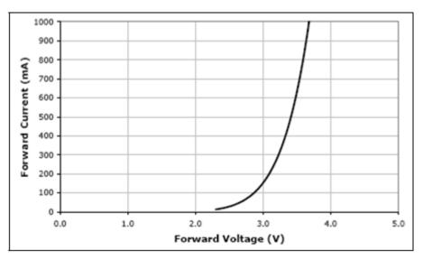
Figure 4. LED Forward Voltage versus Current
