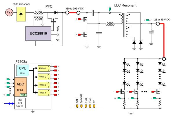
Figure 8. AC LED Lighting and Communications Board Hardware Block Diagram
