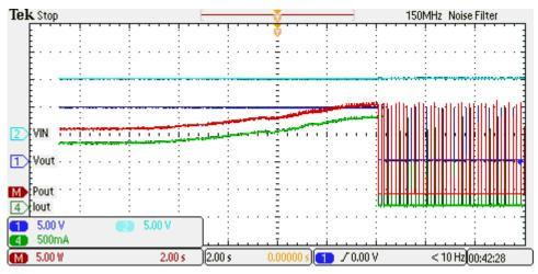
Figure 4: Load Power limited to 15W, for VIN= 10V and Iout is increased from 1A to beyoned 1.5A
