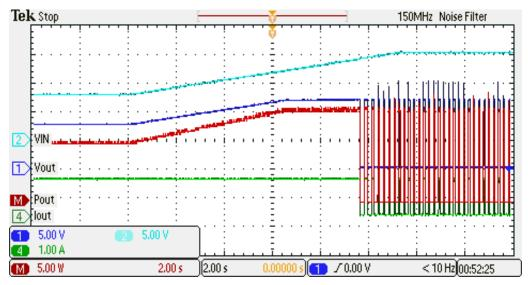
Figure 6 : Load Power limit at 15W, for VIN= 8V to 15V @ 1.1A load
