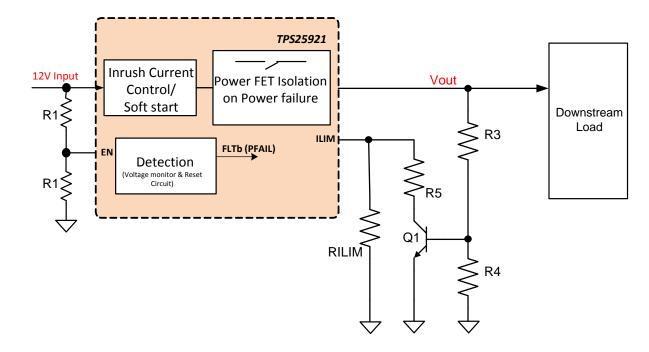
Figure 1: Block Diagram Precision Power Limiting Solution
