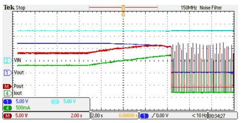
Figure 3: Load Power is limited to 15W for VIN= 12V, Iout varied from 1 to beyond 1.25A
