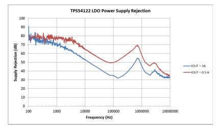
Figure 7. Power Supply Ripple Rejection
