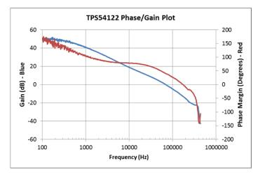
Figure 6. Loop gain and phase
