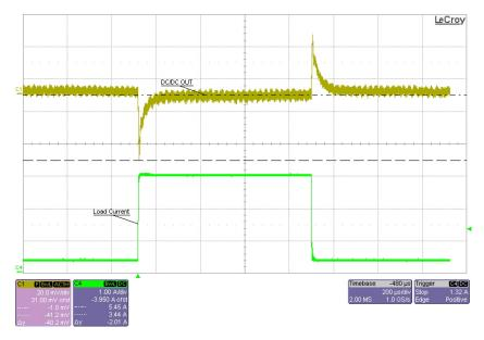
Figure 4. 1.2 V DC/DC Output Transient Response
