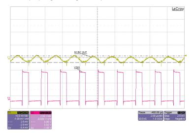
Figure 5. Output ripple and switch node.
