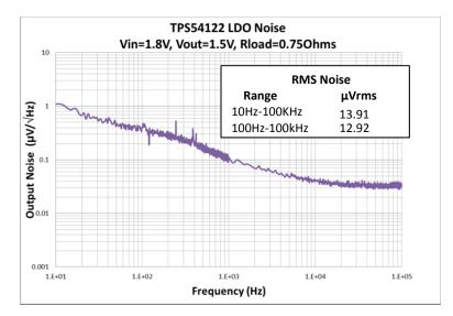
Figure 8. Output Spectral Noise Density (10 Hz to 100 kHz)
