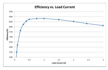
Figure 3. 1.2V DC/DC Output Efficiency
