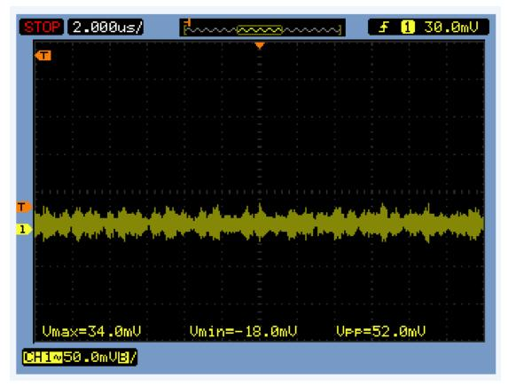
LP38500SD-ADJ: VIN = 5V, VOUT = 3.3V, IOUT = 1.35A Output Ripple Voltage
