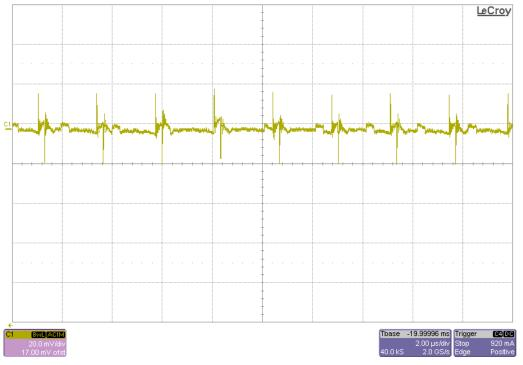
The images below shows the output voltage ripple when load is fully applied. The input voltage is 12V.
