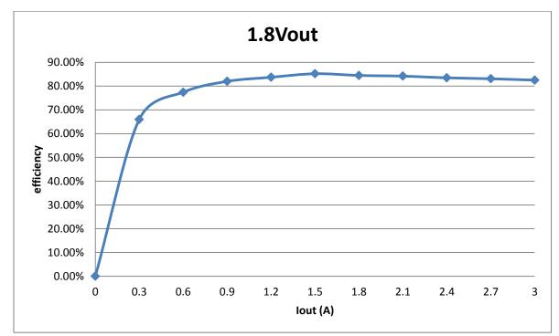
Figure 7. VIN = 12V, VCCAUX Efficiency
