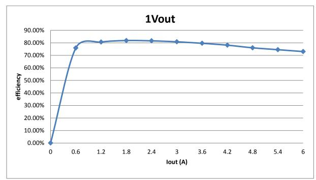
Figure 6. VIN = 12V, VCCINT Efficiency
