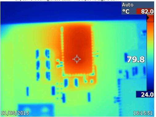
Thermal images at full load of each device are shown below, the remaining rails are not drawing any current during these tests. The input voltage is 12V.
