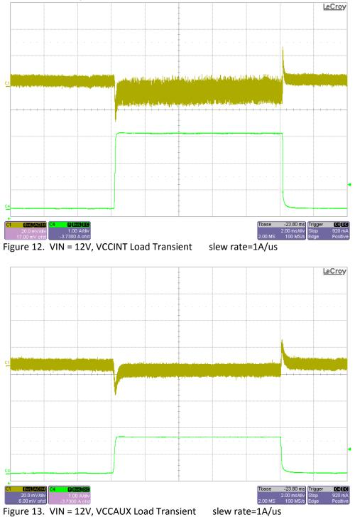
The transient response of the converters is shown below. The input voltage is 12V. The output current is pulsed from 0 to 50% load.
