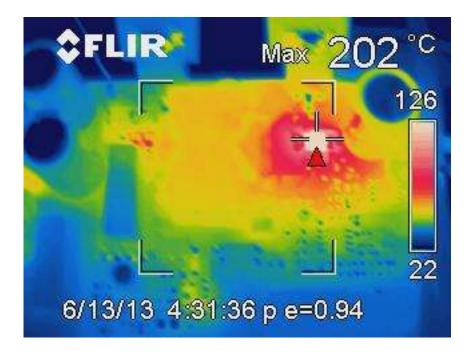
Image taken at full load in still air at 24 deg C. the hottest part on the board is the load current sense R at 202 deg C. Customer should consider a smaller value to reduce this power disappation (2<sup>2</sup>\*.24=.96 watts)
