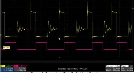
Figure 8. Secondary Side Switching Waveform
