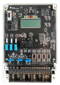
Figure 15. Top View of the Three Phase Energy Meter EVM
