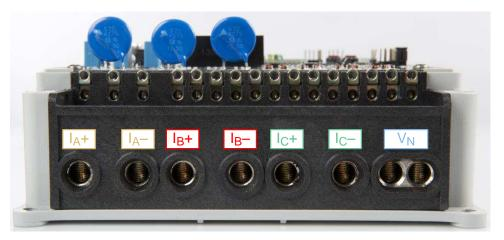
Figure 18. Front View of the EVM With Test Setup Connections
