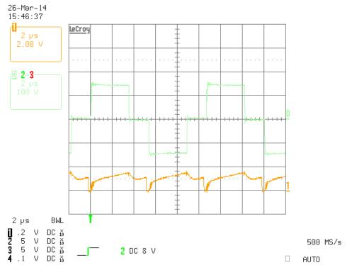
Voltage across the Tx and the current sense pin of the IC at full load
