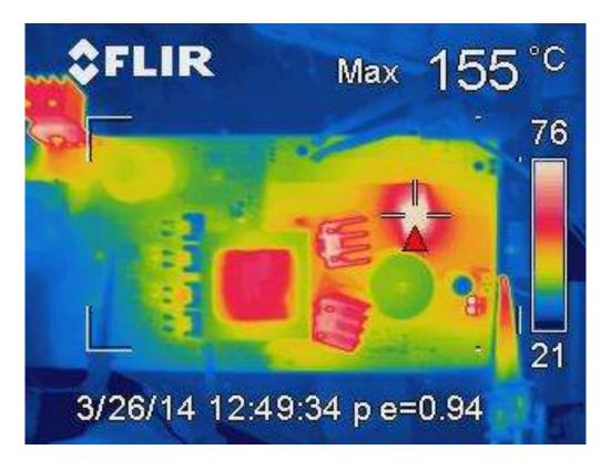
Image taken at full load in still air at 24 deg C. the hottest part on the board is are the snubber Rs and the diode bridge.
