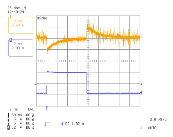
Blue is the load current step, orange is the output voltage response
