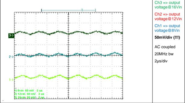
Figure 17, continuous output current results in lowest ripple
