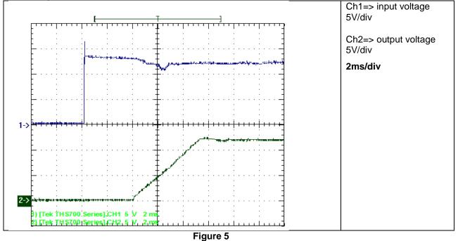
The startup waveform is shown in the Figure 6. The input voltage was set at 12V, with no load at the output.
