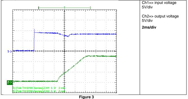
The startup waveform is shown in the Figure 4. The input voltage was set at 12V, with 1.5A load at the output.
