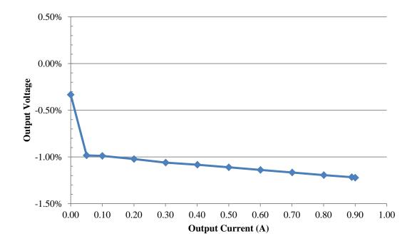
Figure 18 Output regulation of VCCAUX 1.8V output
