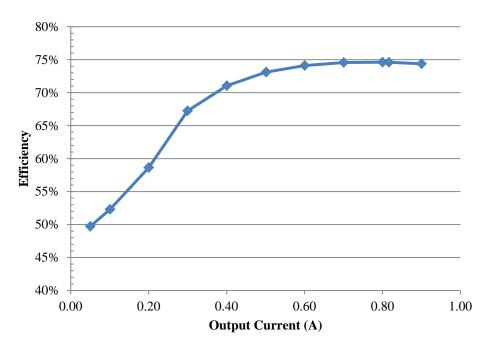
Figure 12 Power efficiency of MGTAVCC 1V output
