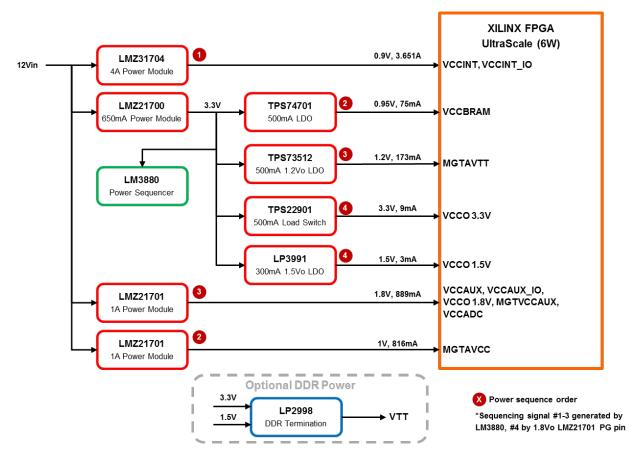
Figure 1 Power supply block diagram
