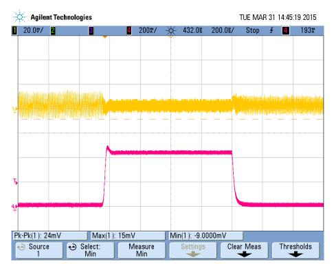
Figure 21 Output load transient of VCCAUX 1.8V output
