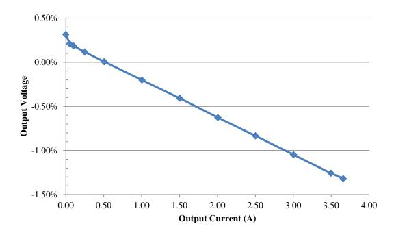
The regulation was measured on three power module outputs, VCCINT 0.9V, MGTAVCC 1V and VCCAUX 1.8V.
