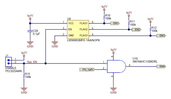
**Figure 4 Power sequencing circuit**
