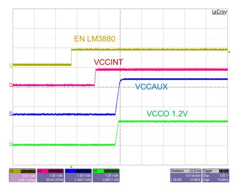
one LM3880 is used for power sequencing as shown in figures 4, 5,
