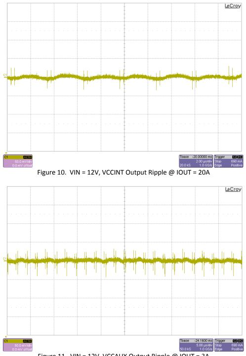
Figure 11. VIN = 12V, VCCAUX Output Ripple @ IOUT = 3A
