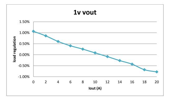
The images below show the output load regulation. The input voltage is 12V.
