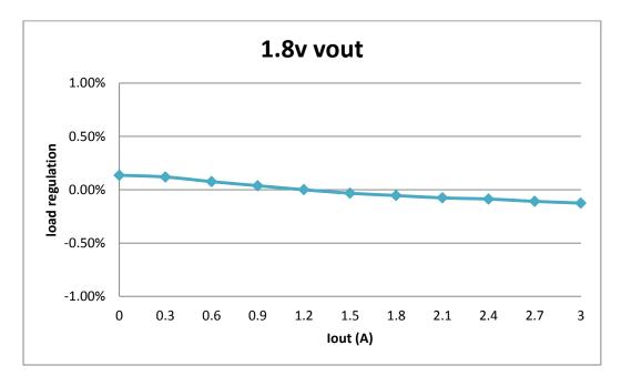
Figure 9. VIN = 12V, VCCAUX Load Regulation
