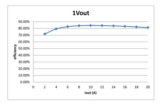
Figure 6. VIN = 12V, VCCINT Efficiency
