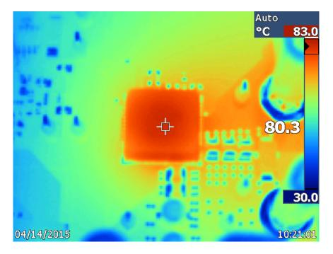
Figure 14. VIN = 12V, VCCINT Thermal Image @ 20A
