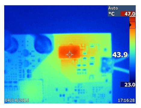
Figure 15. VIN = 12V, VCCAUX Thermal Image @ 3A
