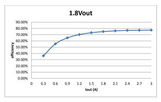
Figure 7. VIN = 12V, VCCAUX Efficiency
