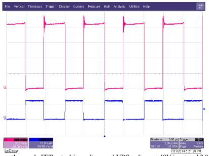
The below waveform shows the synch FET gate drive voltage and VDS voltage at 48V input and 2.9A output current.
