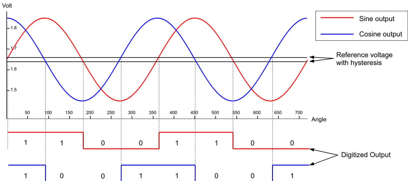
**Figure 4. Quadrature Output Enables Direction Detection**
