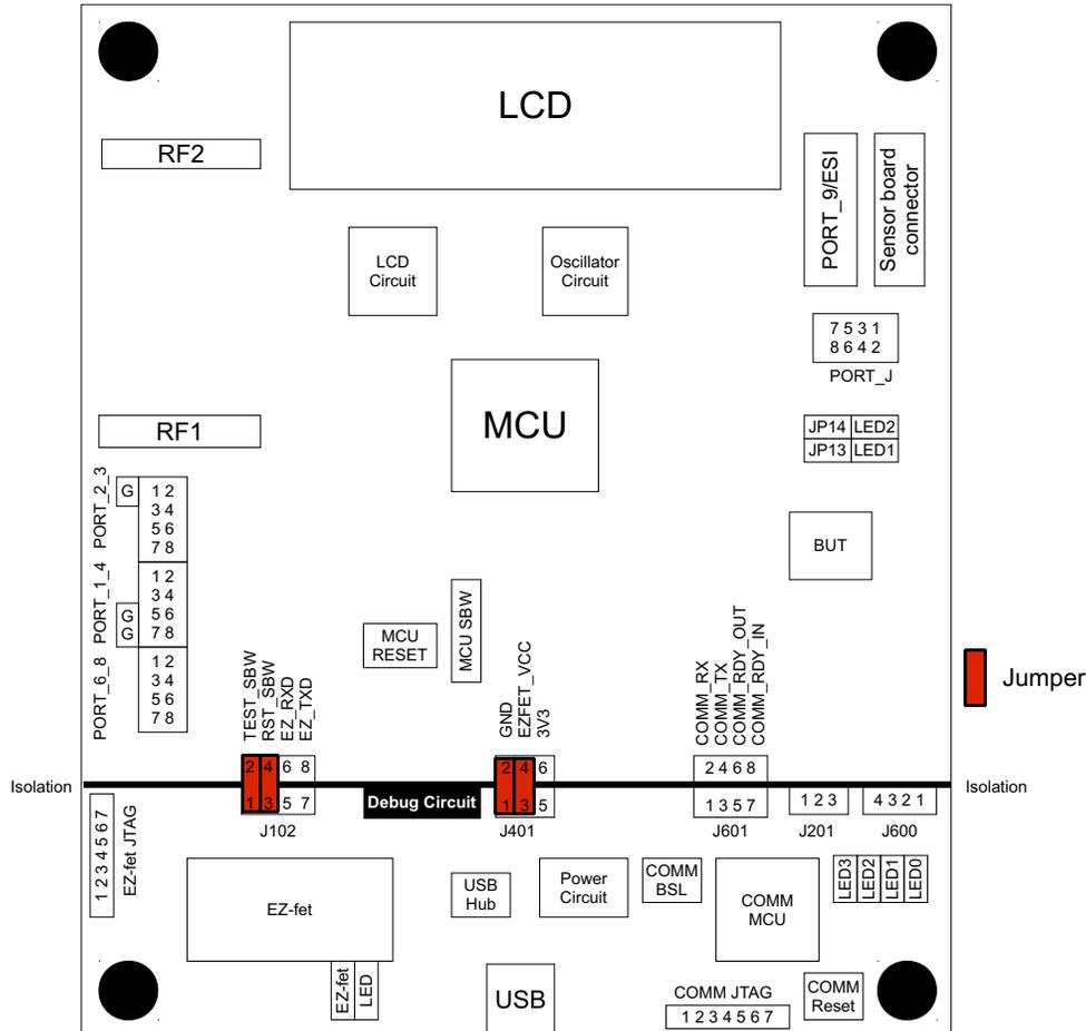
Figure 6. Jumper Setting of Main Board
