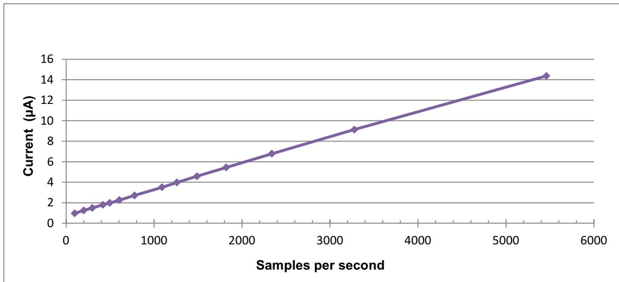
**Figure 8. Power Consumption versus Sampling Rate**
