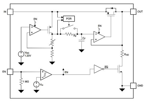
Figure 3: LP5907 Functional block diagram
