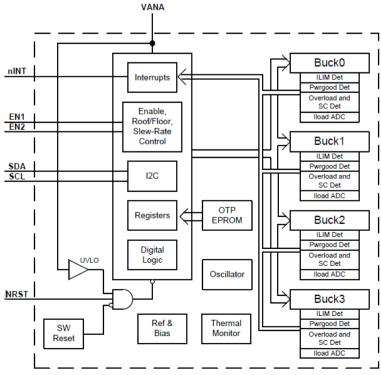
Figure 2: LP8758 Functional Block Diagram
