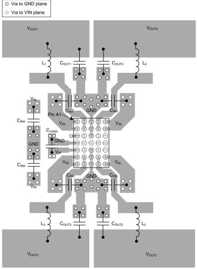
Figure 6: PCB layout example for LP8758
