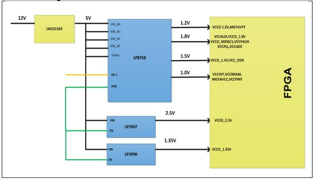
Figure 1 Comprehensive block diagram
