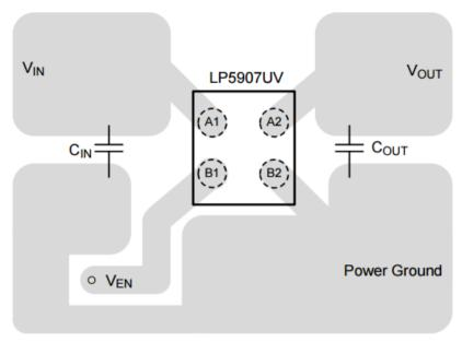
Figure 7: PCB Layout Example for LP5907
