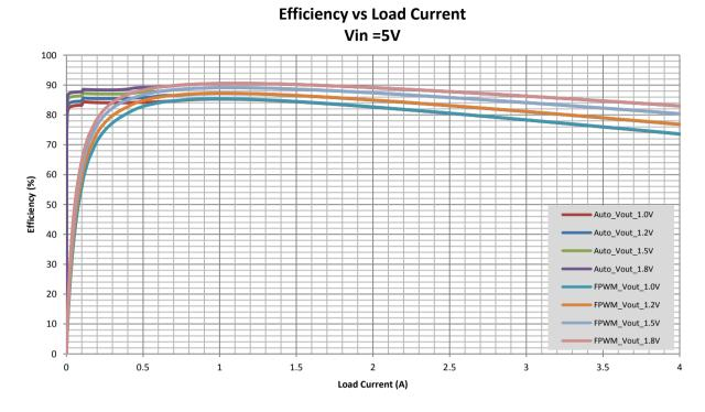
Figure 15: Output Voltage Efficiency in Auto and FPWM Mode
