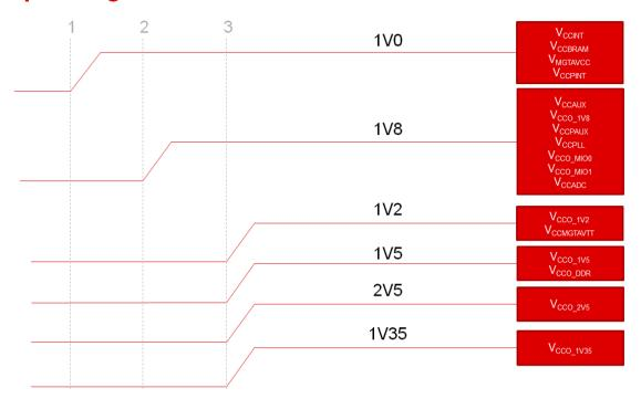
Figure 9 : Example Startup Sequence
