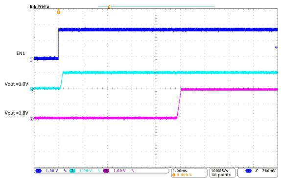
Figure 11: Measured Startup Sequence
