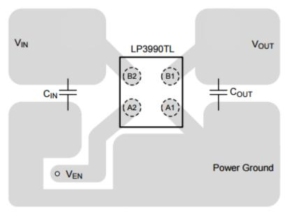
Figure 8 : PCB Layout Example for LP3990
