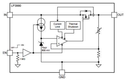
Figure 4: LP3990 Functional Block Diagram
