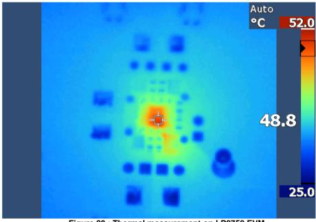
Figure 20: Thermal measurement on LP8758 EVM
