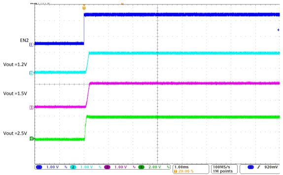
Figure 12: Measured Startup Sequence (Continue)
