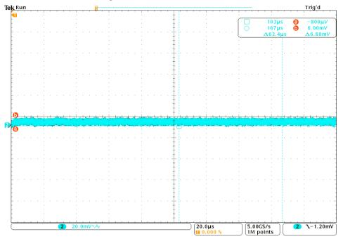
Figure 16: Ripple Voltage at Vout =1.0V
