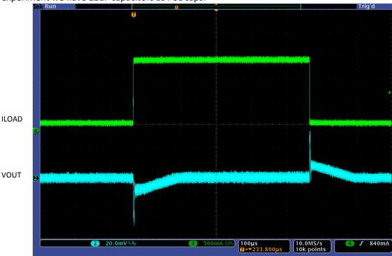
Figure 18: Load Transient for V<sub>OUT</sub> =1.0V with 1A/µsec
