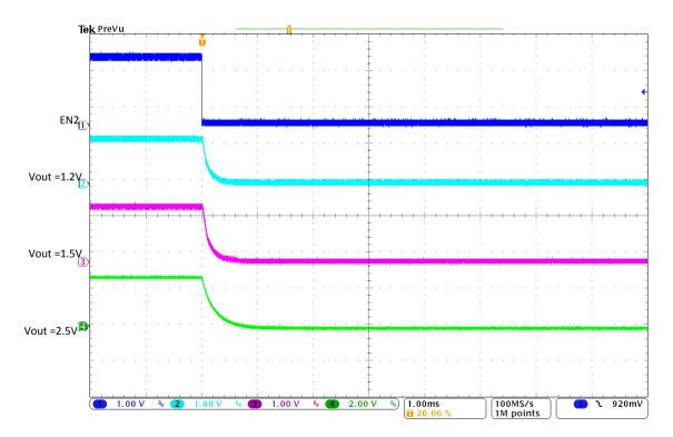
Figure 14: Measured Shutdown Sequence (Continue)
