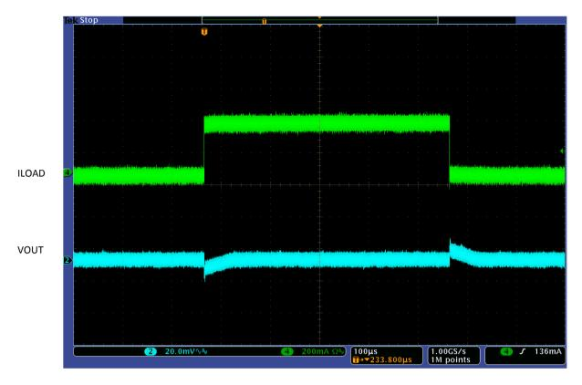
Figure 19: Load Transient for V<sub>OUT</sub> =1.8V with 1A/µsec
