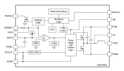
Figure 5: LMZ31503 Functional Block Diagram
