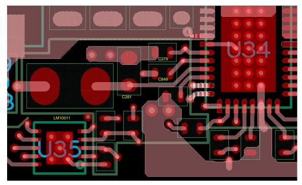
Figure 8. BP3, BP6, VDD Bypass, and LM10011 Position
