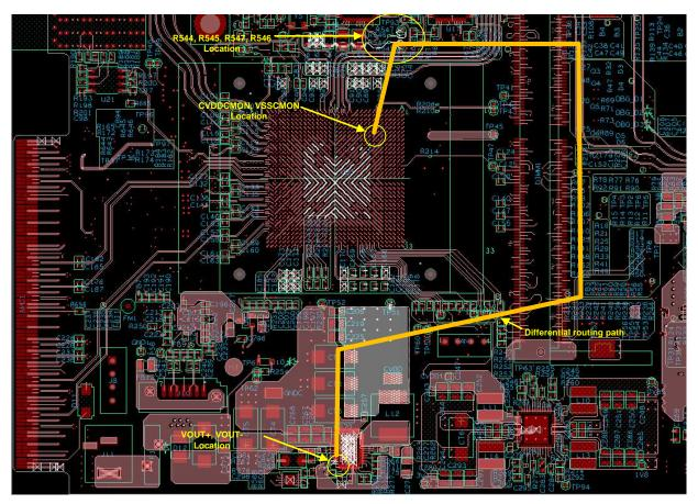
Figure 9. Sense Line Routing
