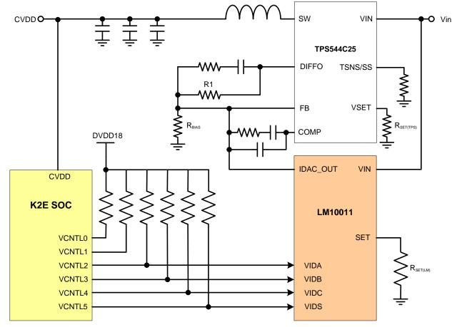
Figure 1. CVDD Power Circuit Using the LM10011 and the TPS544C25
