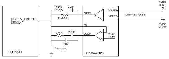
Figure 4. Output Voltage Control Diagram
