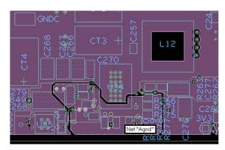
Figure 7. Analog Ground on Layer 2
