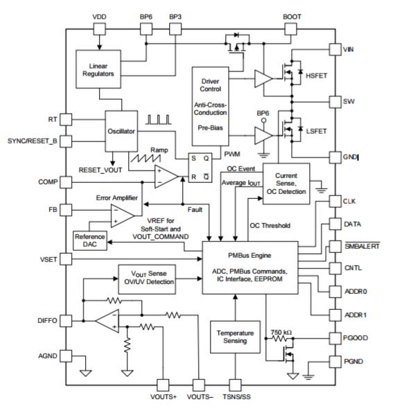
Figure 2. TPS544C25 Functional Block Diagram
