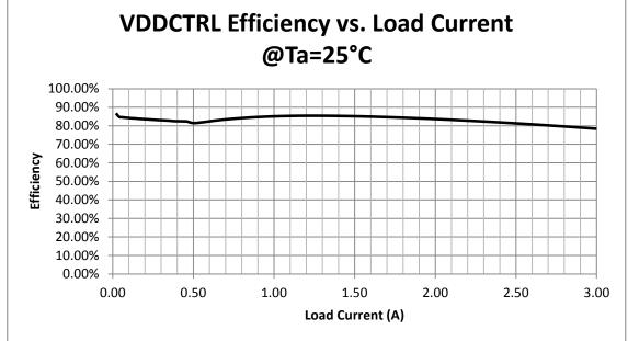
Figure 7 – CTRL1 Efficiency @ 25C
