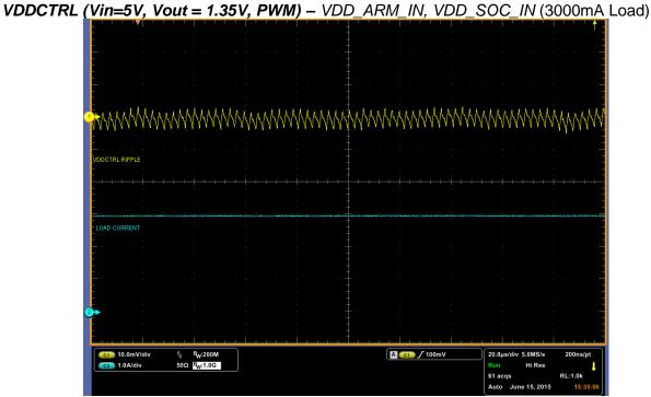
Figure 15 – VDDCTRL Voltage Ripple @ 25C
