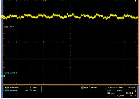
Figure 13 – DCDC2 Voltage Ripple @ 25C
