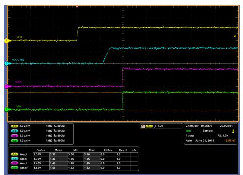
Figure 23 – Power-Up Sequence (No Load) Voltage Waveforms (LDO8\_3.3V, VDDCTRL\_1.35V, VDD1\_1.5V, VIO\_1.5V)
