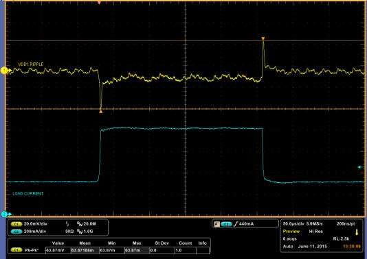
Figure 16 – DCDC1 Load Transient @ 25C
