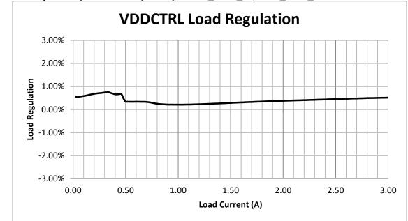
VDDCTRL (Vin=5V, Vout=1.35V, PWM) - VDD\_ARM\_IN, VDD\_SOC\_IN
