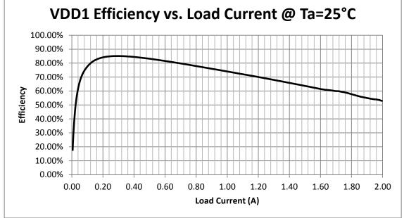
Figure 4 - DCDC1 Efficiency @ 25C
