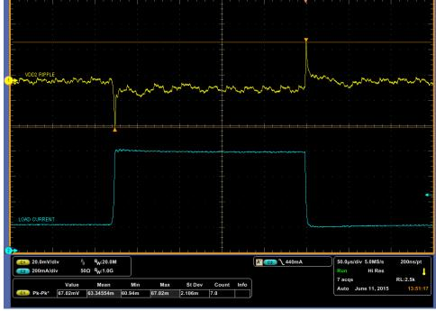
Figure 17 – DCDC2 Load Transient @ 25C
