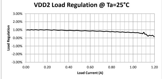
Figure 9 – DCDC2 Load Regulation @ 25C
