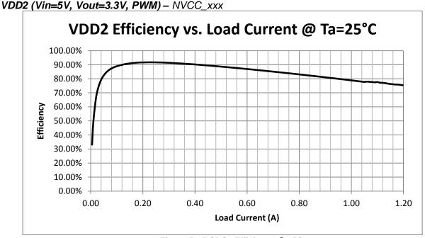
Figure 5 – DCDC2 Efficiency @ 25C
