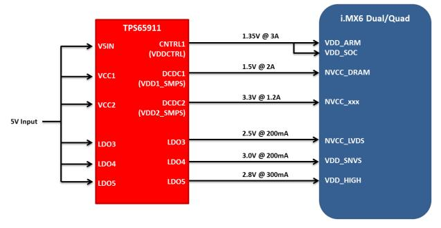
Figure 3 – IMX6 Block Diagram
