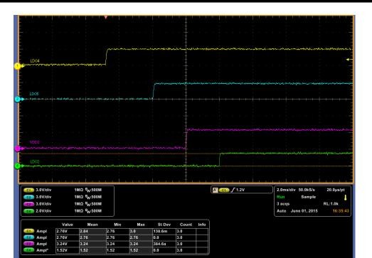
Figure 21 – Power-Up Sequence (No Load) Voltage Waveforms (LDO4\_3.0V, LDO5\_2.8V, VDD2\_3.3V, LDO2\_1.5V)
