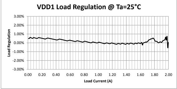
Figure 8 – DCDC1 Load Regulation @ 25C
