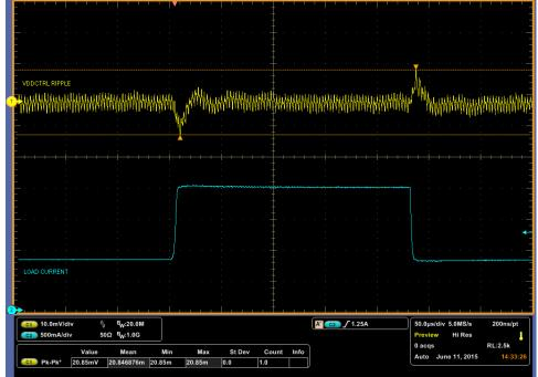
Figure 19 – VDDCTRL Load Transient @ 25C
