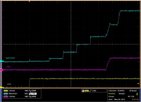
Figure 20 - Power-Up Sequence (Half Max Load) Current Consumption
