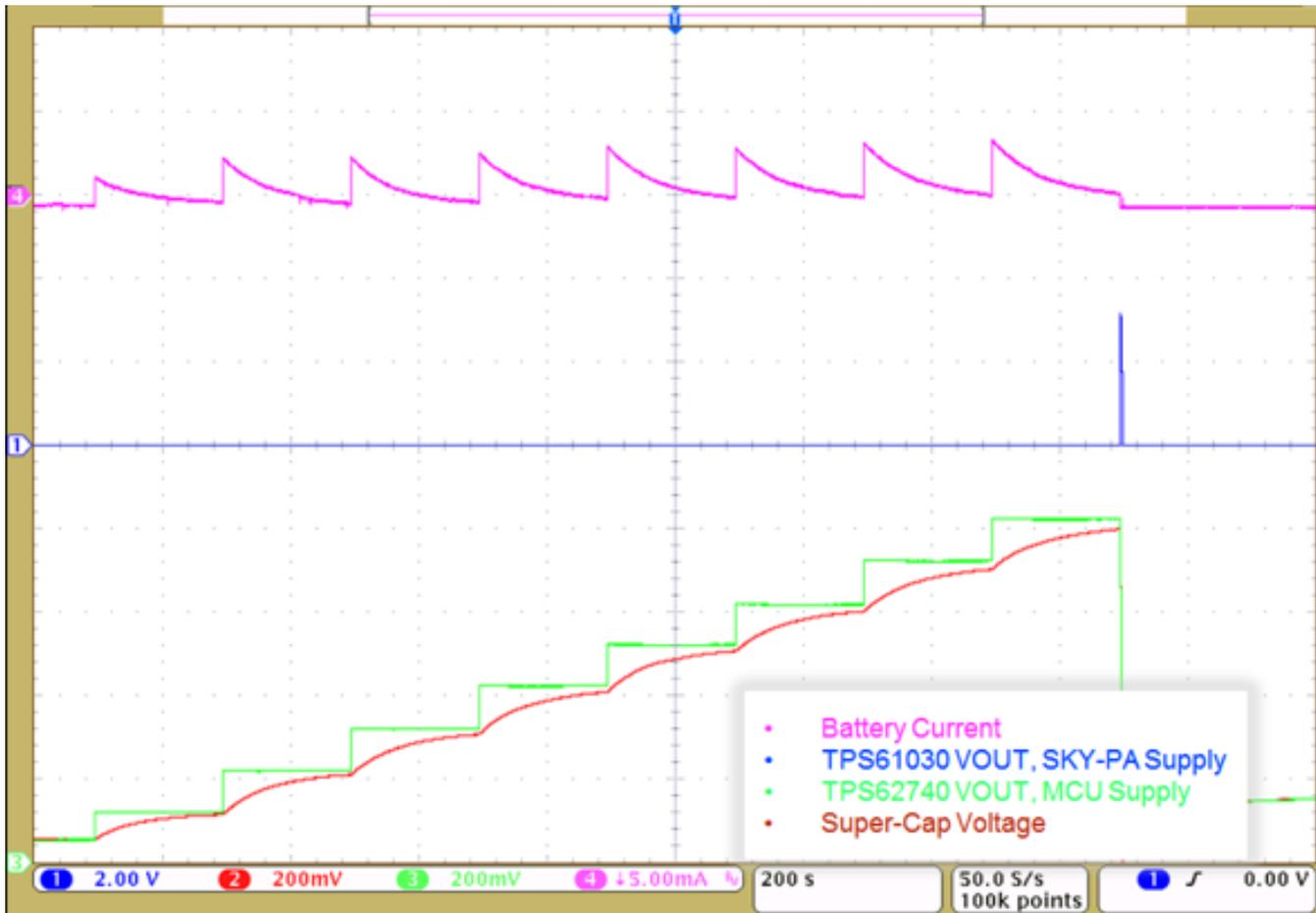
**Figure 10. Transmission Sequence Including Energy Buffering**
