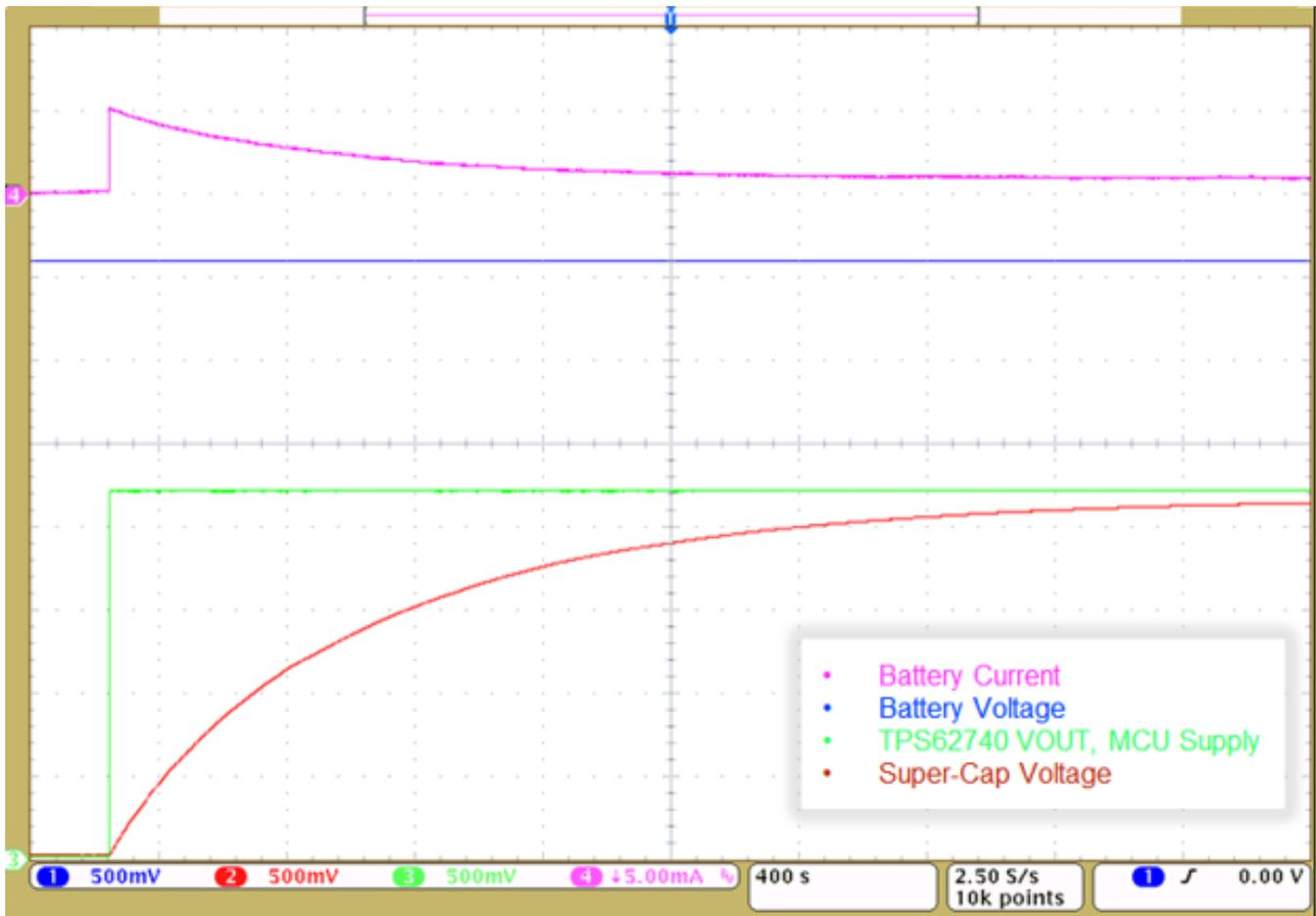
Figure 12. Startup Waveform for Initialization
