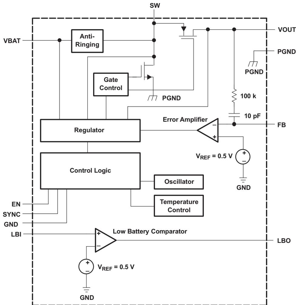
Figure 2. TPS61030 Block Diagram
