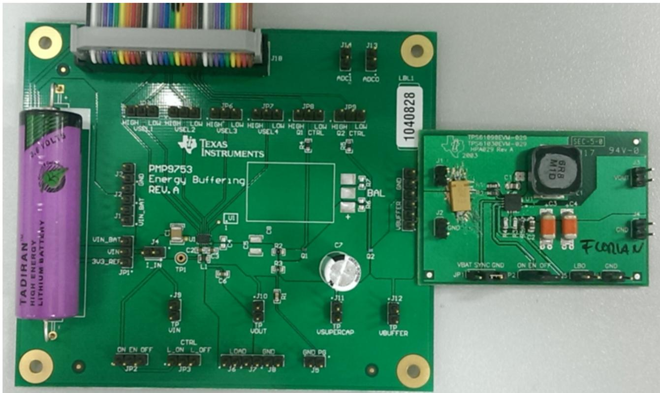
**Figure 7. Power Management Solution (PMP9753 + TPS61030 EVM)**
