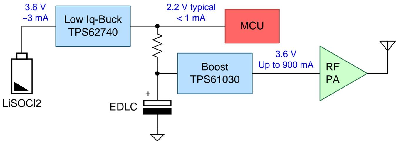
Figure 6. High Current Power Solution for Battery-Operated Meters Block Diagram
