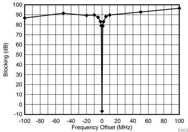
**Figure 15. Ncd Blocking (Measured at Nc Channel)**
