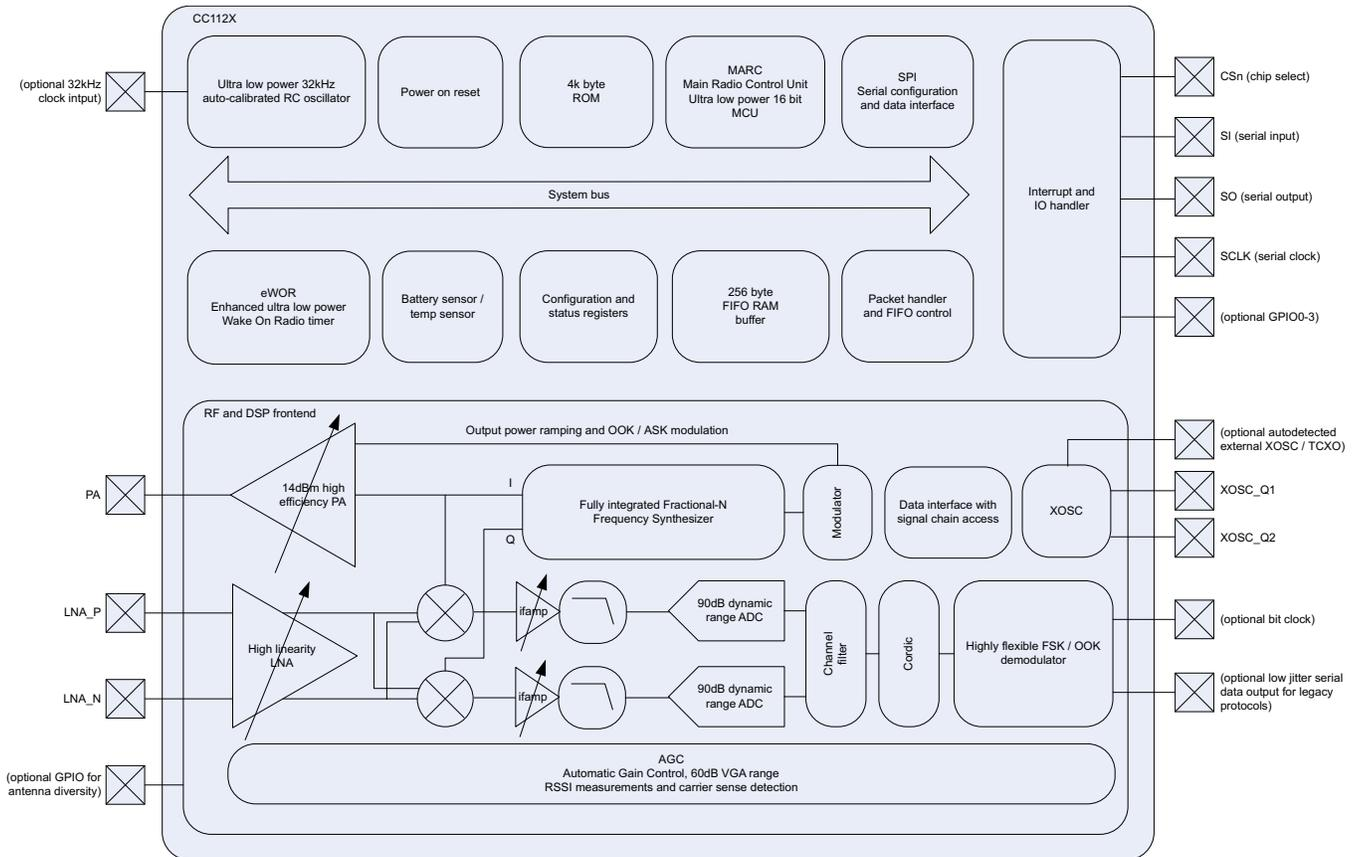
**Figure 4. CC1120 Functional Block Diagram**
