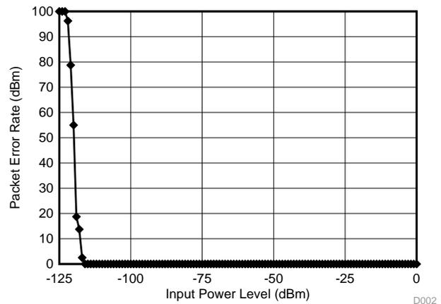
**Figure 14. Nabef PER Plot (Measured at Na Channel)**
