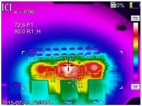
FET temperature: 80°C; Inductor temperature:72.8°C. (Test conditions: 12Vin, 1.085V/90A, 300kHz, 200LFM, Room Temperature.)
