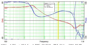
10Vin, 1.0Vout, 90A Load, BW=50.9kHz, PM=81deg, GM=25dB
