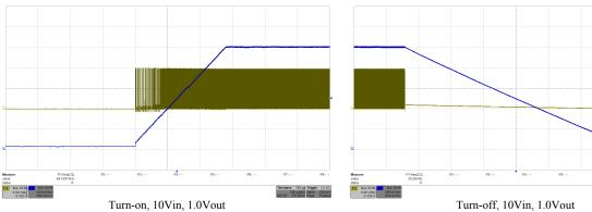
(blue trace is Vout and yellow trace is switching waveform)
