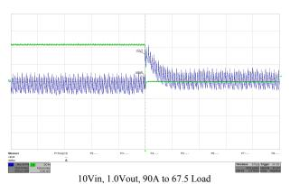
(blue trace is Vout, 10mV/div and green trace is step current 10A/div)
