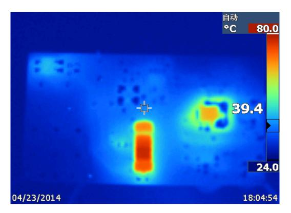
Soldering side, 115Vac at Full Load, Ta=25 $^\circ\,$  C
