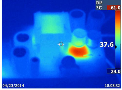
Component side, 115Vac at Full Load, Ta=25° C
