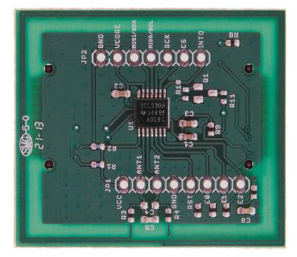
Figure 2. RF430CL330HTB Target Board
