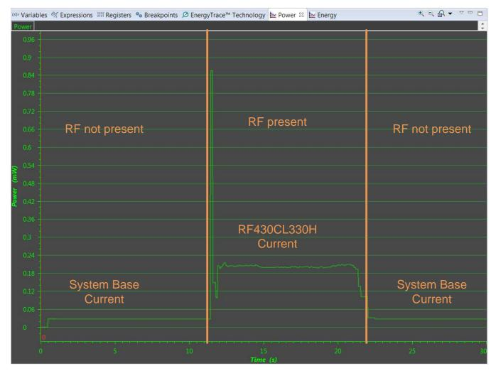
Figure 10. Power Profile of 30-Second Measurement at 3.3-V Power Supply
