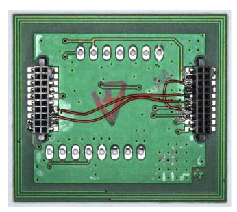
Figure 5. RF430CL330HTB Bottom View
