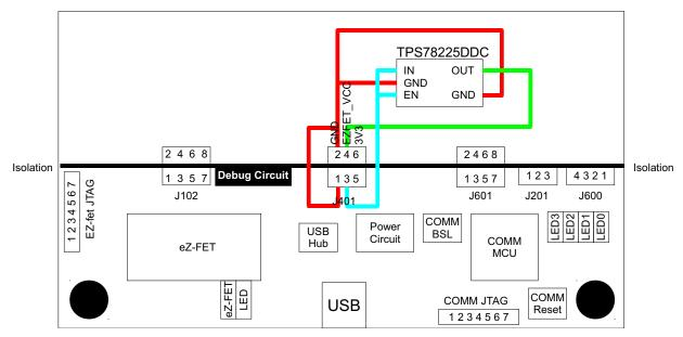
Figure 11. Voltage Regulator Connection on the EVM430-FR6989 Main Board
