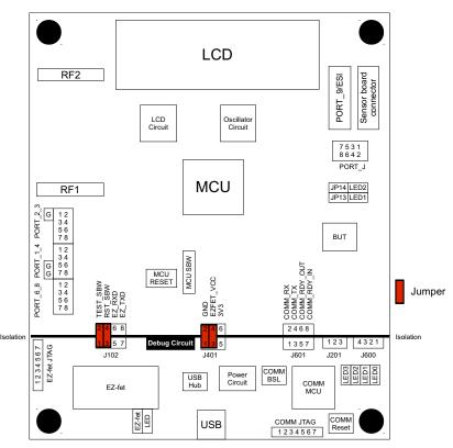
Figure 8. Jumper Setting of Main Board
