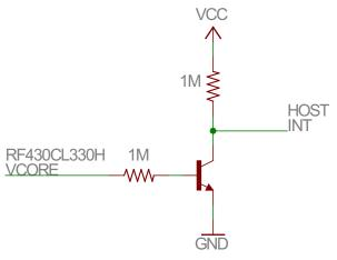
Figure 3. Wake Circuit
