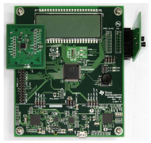
Figure 7. EVM430-FR6989 Main Board With RF430CL330HTB Target Board Attached
