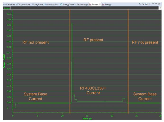
Figure 12. Power Profile of 30-Second Measurement at 2.5-V Power Supply
