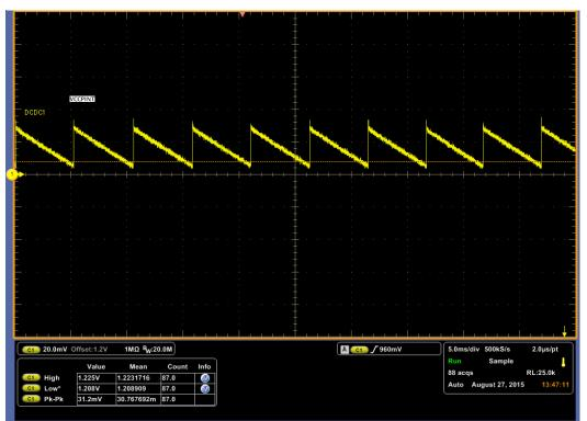
Figure 10 – DCDC1 Voltage Ripple, Light Load @ 25C
