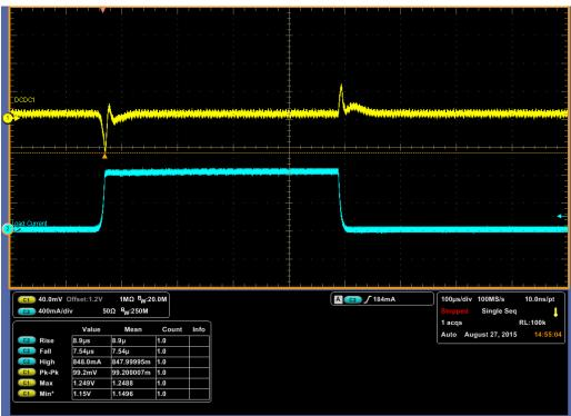
Figure 16 – DCDC1 Load Transient Response @ 25C
