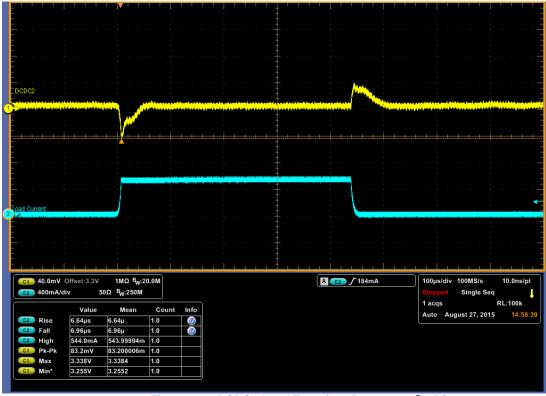
Figure 17 – DCDC2 Load Transient Response @ 25C
