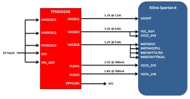
Figure 3 – Spartan 6 Block Diagram
