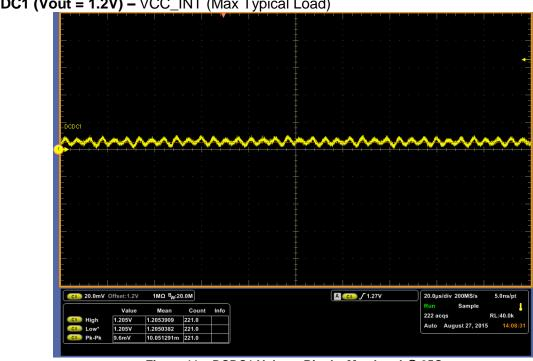
DCDC1 (Vout = 1.2V) - VCC\_INT (Max Typical Load)
