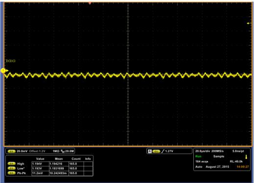
Figure 15 – DCDC3 Voltage Ripple, Max Load @ 25C
