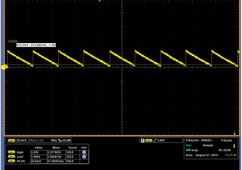
Figure 12 – DCDC2 Voltage Ripple, Light Load @ 25C
