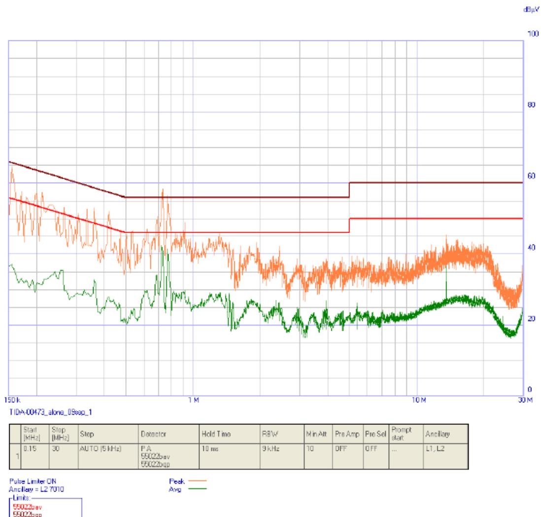
Figure 21. Conducted Emissions as per EN55022 Class B
