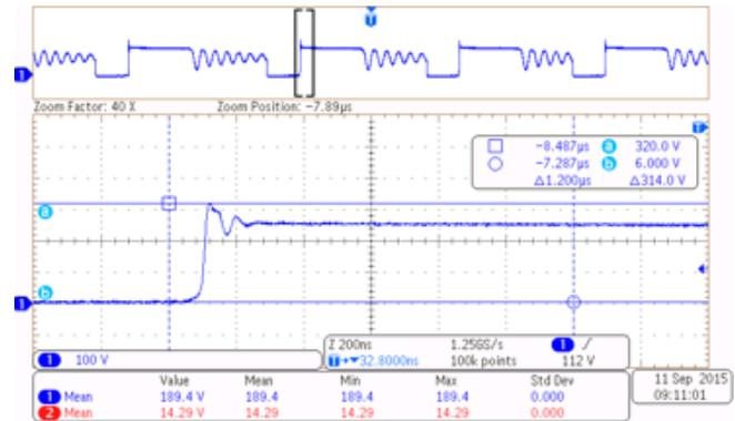
Figure 12.  $V_{DS}$  Waveform at  $V_{IN} = 115$ -V AC, Full Load
