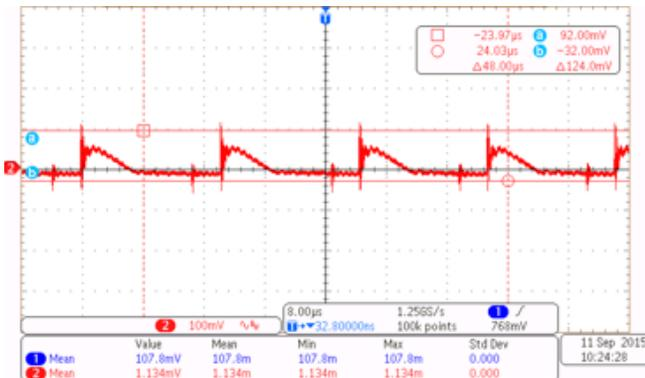
Figure 15. 10-V Output Voltage Ripple at Full Load
