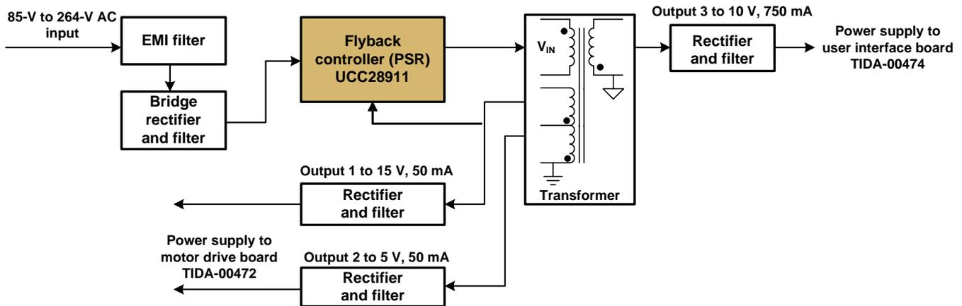
Figure 1. Block Diagram of Power Supply With Isolated Multiple Outputs
