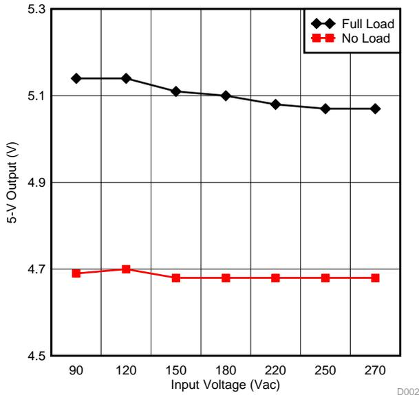
Figure 7. Line Regulation at 5-V Output With Full Load and No Load
