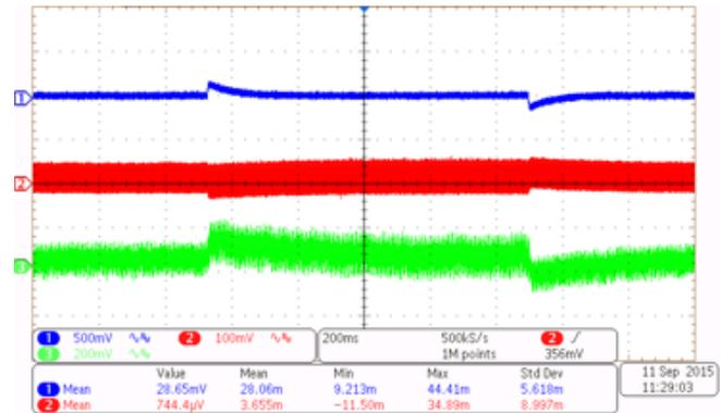
Figure 19. Step Load at 15-V Output (0 to 0.05 A)
