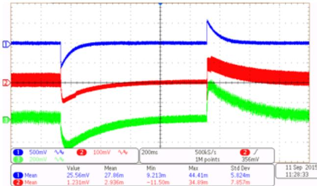
Figure 18. Step Load at 10-V Output (0.1 to 0.75 A)
