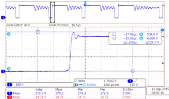
Figure 11.  $V_{DS}$  Waveform at  $V_{IN} = 270$ -V AC, Full Load
