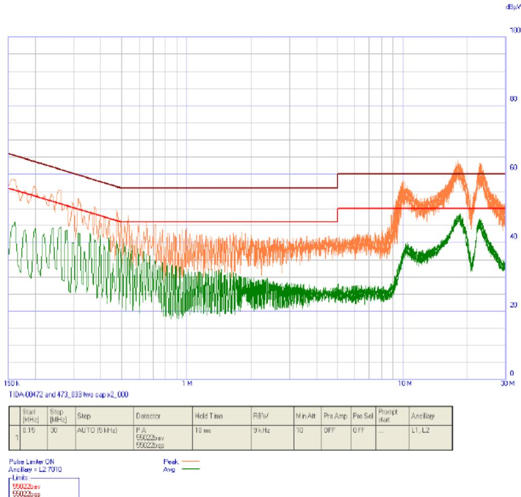
Figure 22. Conducted Emissions as per EN55022 Class B (TIDA-00473 and TIDA-00472 Connected Together)
