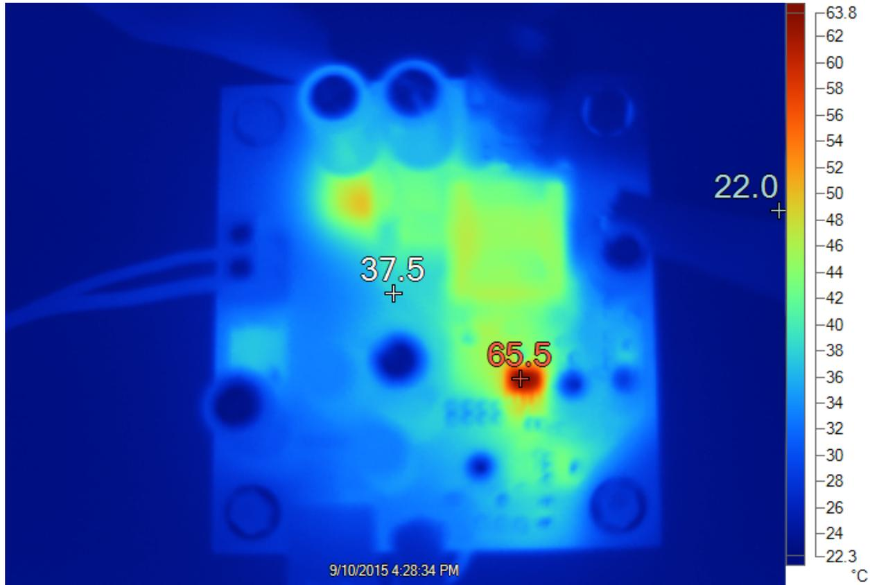
**Figure 23. Top Side Temperatures at 90-V AC, 10.4-W Input Power**
