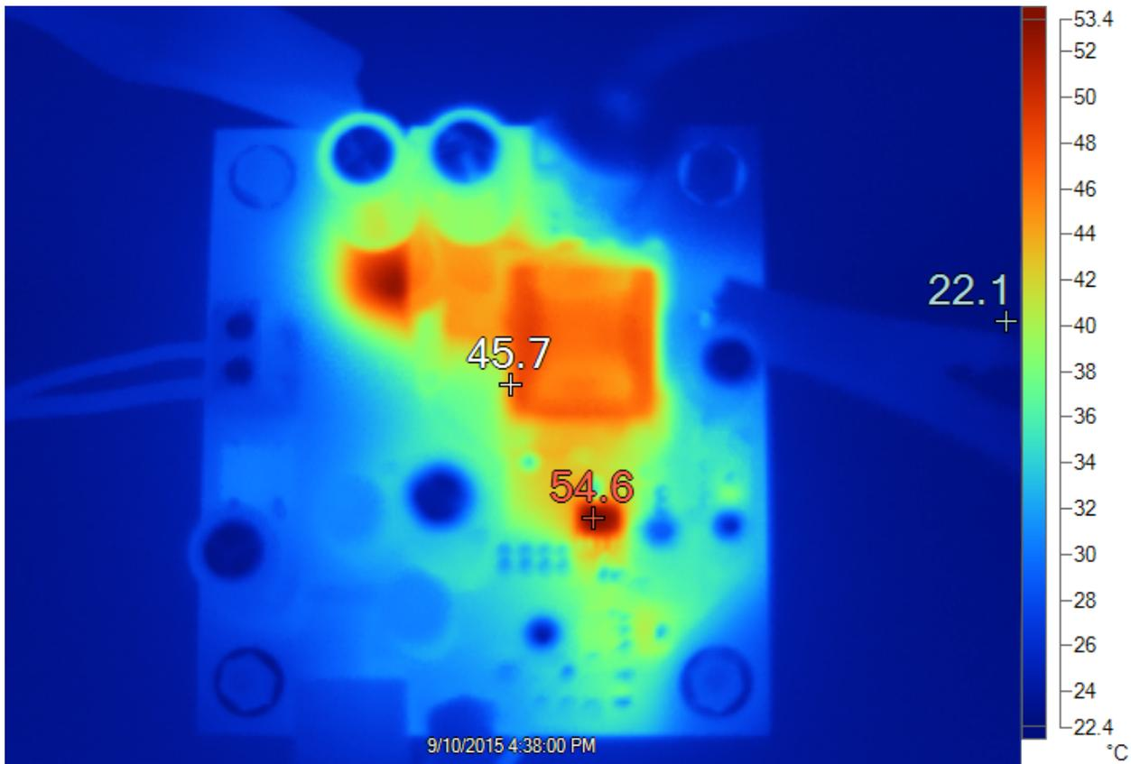
**Figure 24. Top Side Temperatures at 230-V AC, 10.4-W Input Power**
