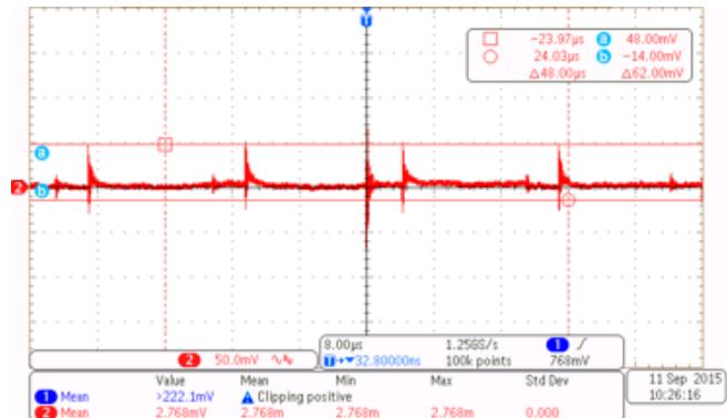
Figure 16. 15-V Output Voltage Ripple at Full Load
