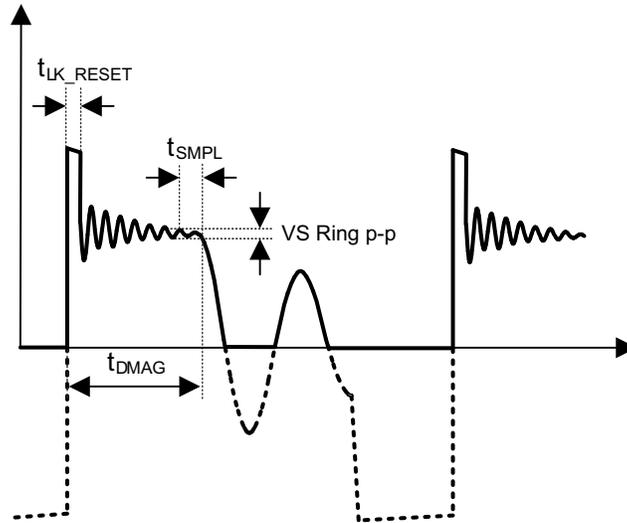
Figure 3. VS Voltage
