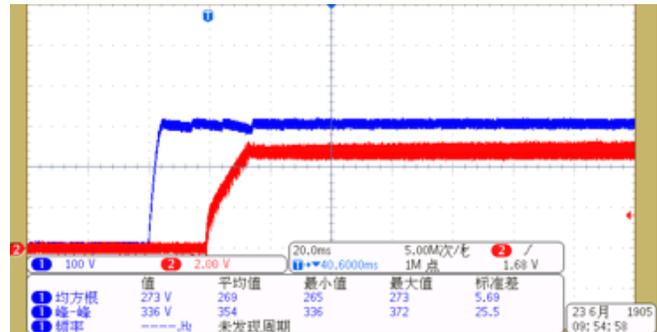
Figure 14. Start-up Time Under 230-V AC Input
