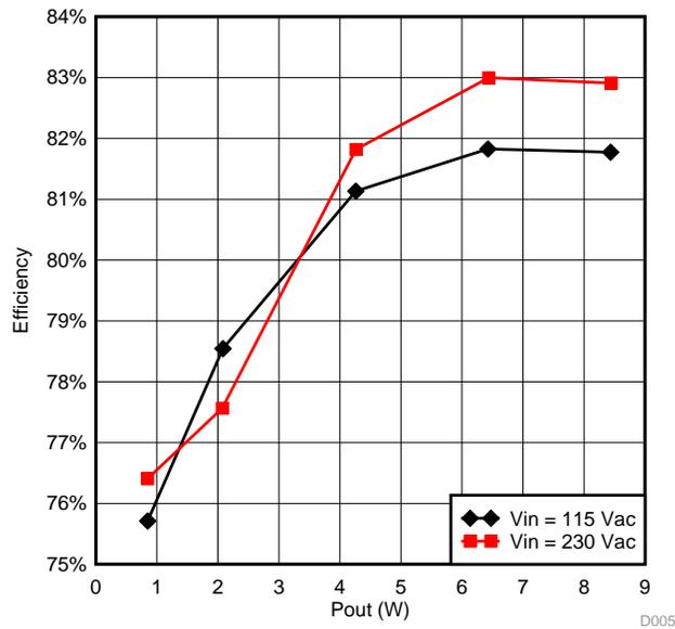
Figure 10. Efficiency Curves at 115-V AC and 230-V AC Inputs
