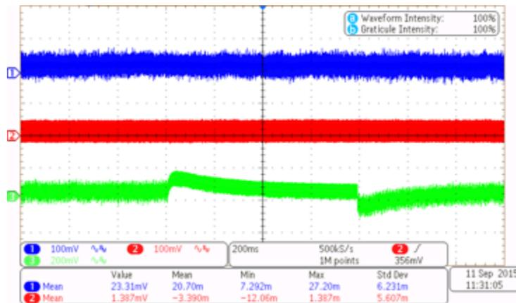
Figure 20. Step Load 5 V (0 to 0.05 A)
