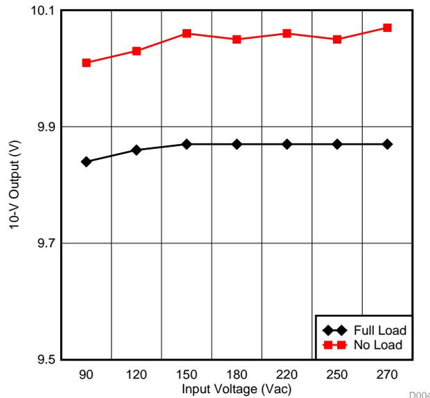
Figure 9. Line Regulation at 10-V Output With Full Load and No Load
