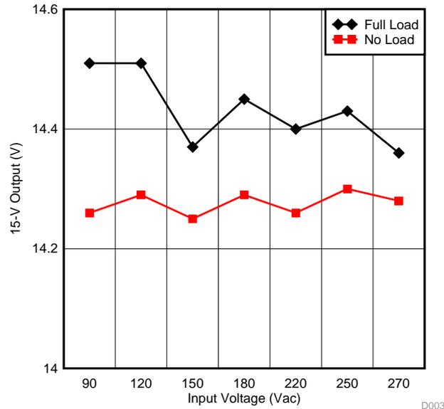
Figure 8. Line Regulation at 15-V Output With Full Load and No Load
