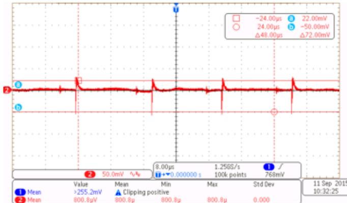
Figure 17. 5-V Output Voltage Ripple at Full Load
