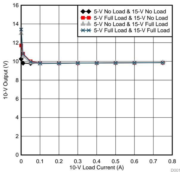
**Figure 6. Cross Regulation at 10-V Output With 5-V and 15-V Load Parameter**
