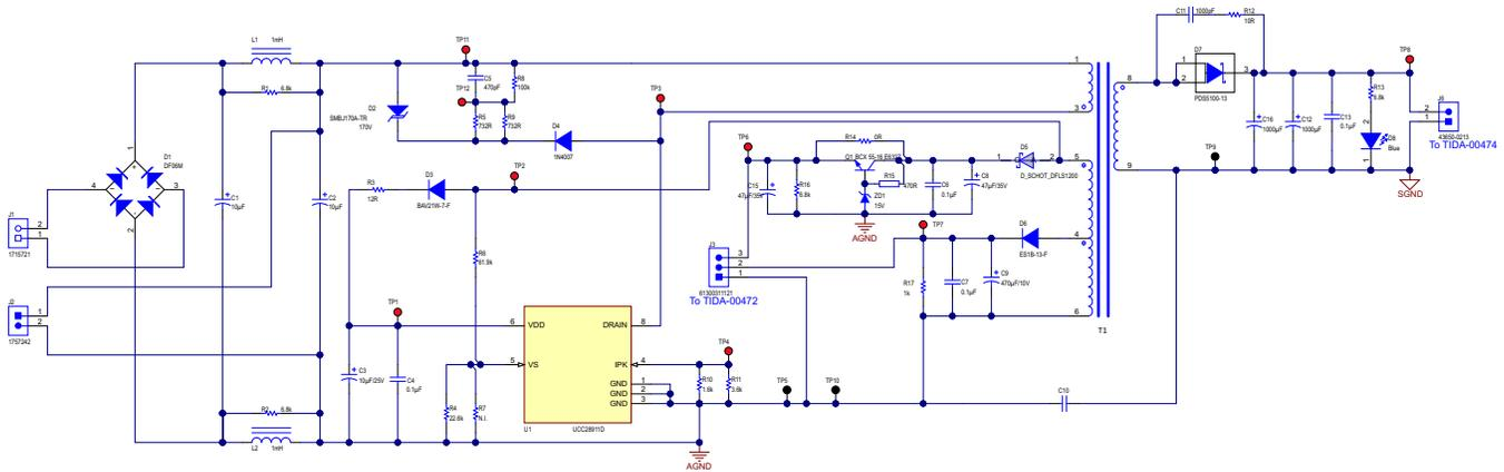
**Figure 2. Multiple Output Flyback Converter Based on UCC28911**
