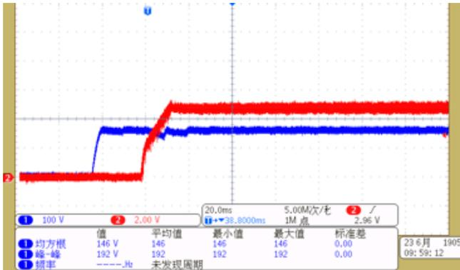
Figure 13. Start-up Time Under 115-V AC Input
