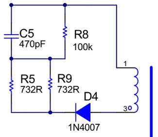
**Figure 4. Drain Clamp Circuit Options**
