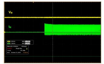
Figure 2. V<sub>M</sub> Stable with Current Limiting
