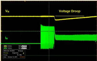
**Figure 1.** V<sub>M</sub>Droop Without Current Limiting
