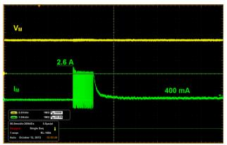
Figure 6. Startup and Steady State Current
