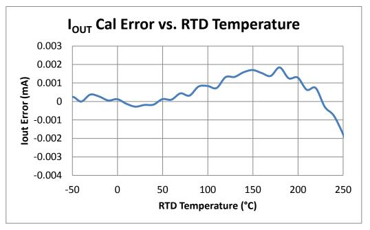
Figure 16: Calibrated Output Current Error vs. RTD Temperature
