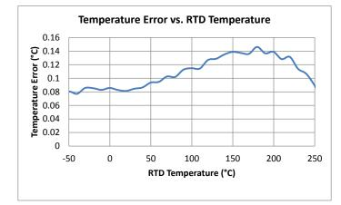
Figure 1: Measured Unadjusted Temperature Error
