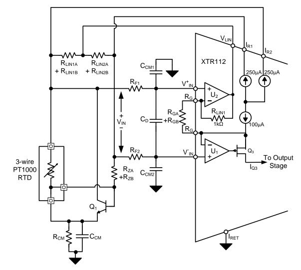
Figure 4: XTR112 Input Excitation, Linearization, and Amplification Stage
