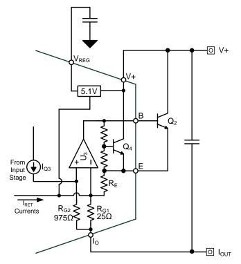
Figure 5: XTR112 Current Loop Transmitter Circuitry
