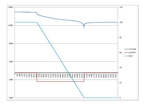
Cell configuration: 4S1PDischarge current: 2500mA
