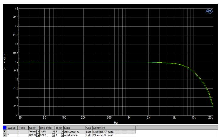
Frequency Response 1W 40hms (Measurement setup uses 20KHz cutoff)
