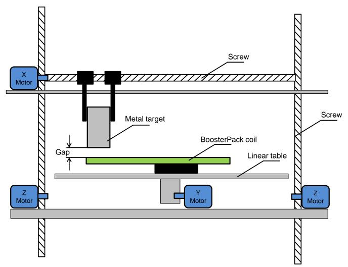
Figure 16. Raw Data Collection Setup
