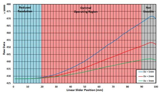
Figure 22. LDC1612 Raw Data Versus Linear Position
