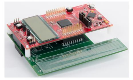
Figure 11. Inductive Linear Position Sensing Reference Design
