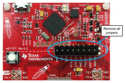
Figure 18. External Power Supply Jumper Configuration
