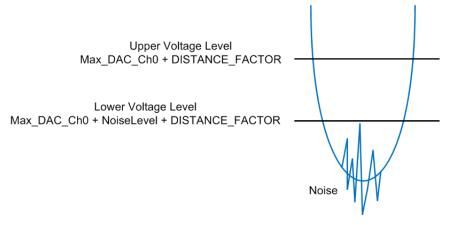
Figure 15. Optimal DAC Setting
