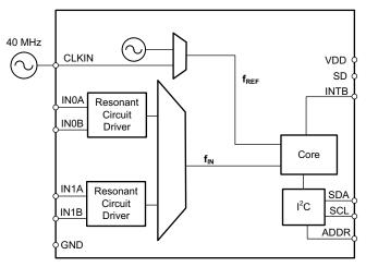
Figure 5. Functional Block Diagram of the LDC1612
