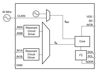
Figure 2. LDC1612 Block Diagram
