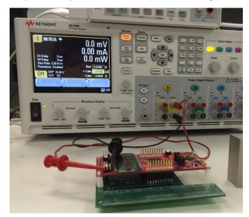
Figure 19. DC Power Analyzer Power Consumption Test Configuration
