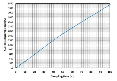
Figure 25. System Power Consumption for LDC Mode
