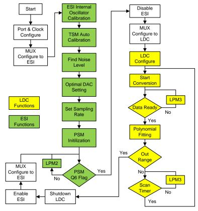
Figure 13. Flowchart of the Firmware
