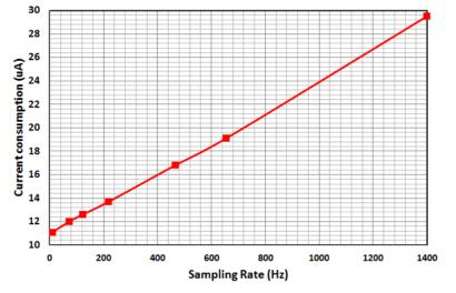
Figure 24. System Power Consumption for ESI Mode
