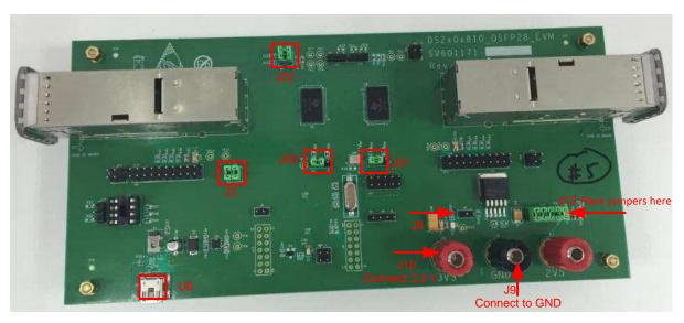
Figure 1. 3.3-V Mode Connections
