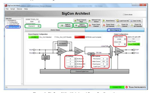
Figure 9. SigCon GUI—High Level Page Configuration
