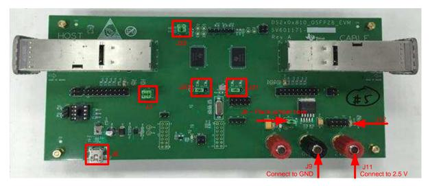
Figure 2. 2.5-V Mode Connections
