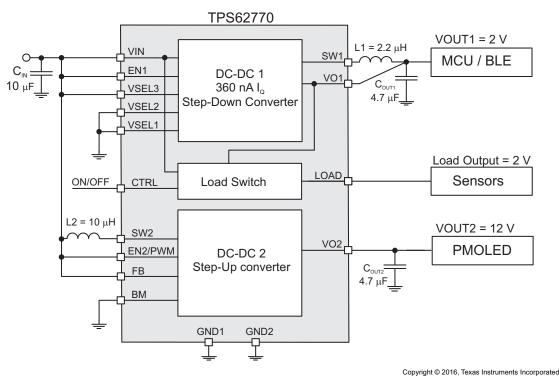
Figure 2. TPS62770 Internal Block Diagram
