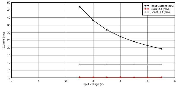
Figure 9. Current Consumption Measurements
