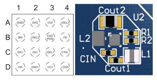
Figure 7. TPS62770 Device Pinout and Layout
