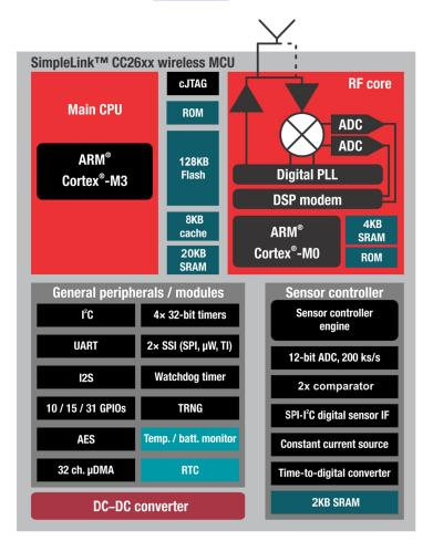
Figure 3. CC2650 Internal Block Diagram
