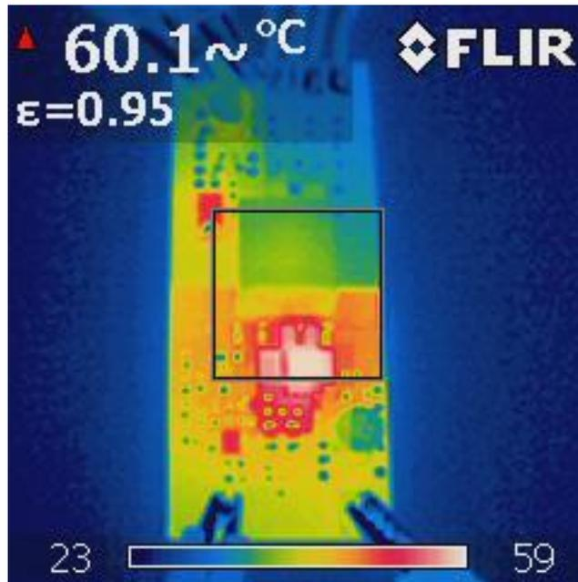
**IR thermal image taken at steady state at 100% load and  $V_{IN} = 15\text{ V}$  (secondary control) for two minutes with no airflow (4 Layer board, 1 Oz copper layer)**
