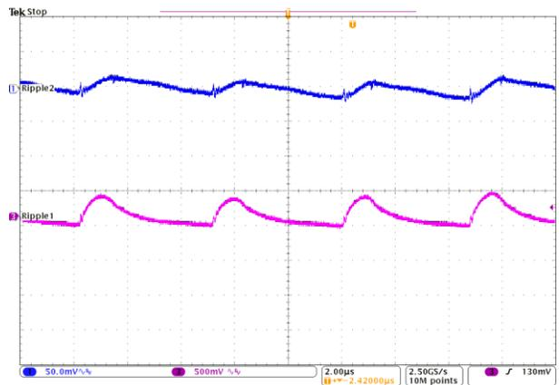
$V_{IN}=15V, I_1=0.1A; I_2=0.1A; I_3=0.5A$
