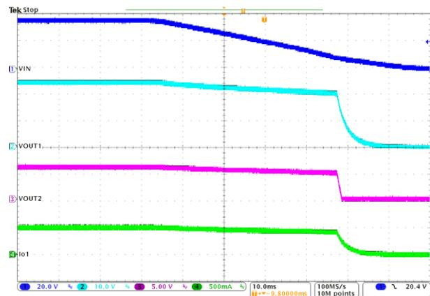
$V_{IN}=36V, I_1=0.1A; I_2=0.1A; I_3=0.5A$
