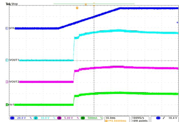
$V_{IN}=36\text{V}$ ,  $I_1=0.1\text{A}$ ;  $I_2=0.1\text{A}$ ;  $I_3=0.5\text{A}$
