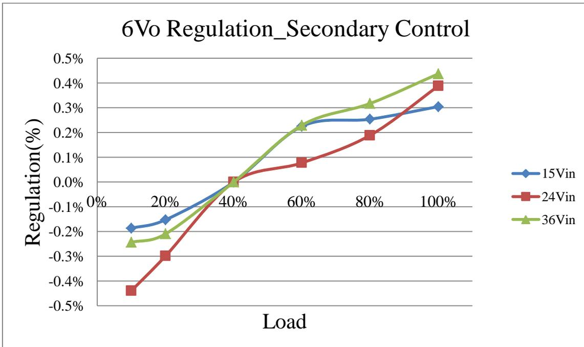
The regulation under unbalanced load was tested by sweeping different load current on the 24V output while the two +6V output were loaded with 10mA, 50mA and 100mA at 24V input. Since the two +6V outputs are symmetrical, only one rail output regulation is shown.
