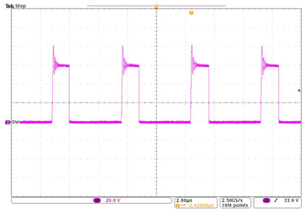
$V_{IN}=15V, I_1=0.1A; I_2=0.1A; I_3=0.5A$
