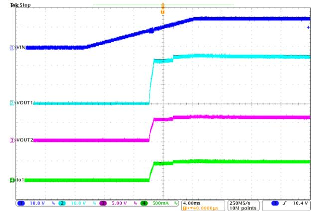
$V_{IN}=15\text{V}$ ,  $I_1=0.1\text{A}$ ;  $I_2=0.1\text{A}$ ;  $I_3=0.5\text{A}$
