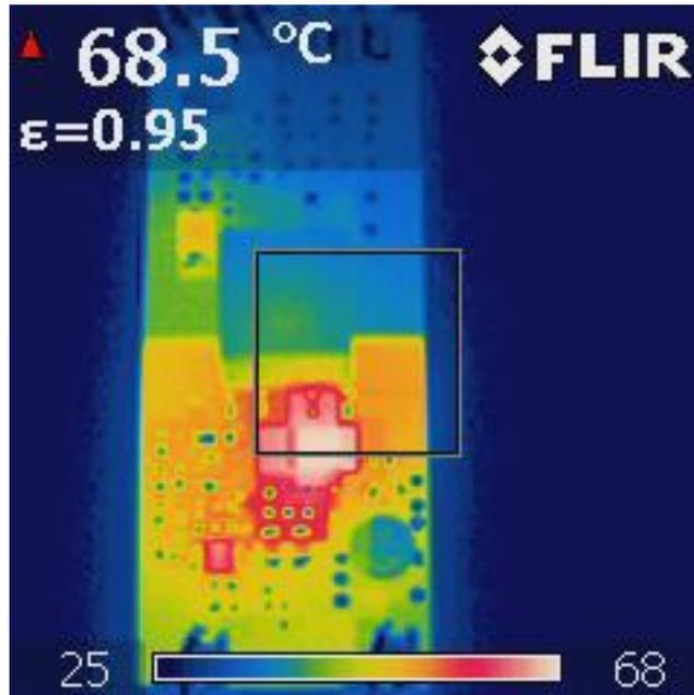
**IR thermal image taken at steady state at 100% load and  $V_{IN} = 36\text{ V}$  (secondary control) for two minutes with no airflow (4 Layer board, 1 Oz copper layer)**
