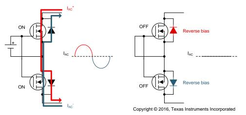
Figure 9. Functionality of MOSFETs for (Left) ON and (Right) OFF Times
