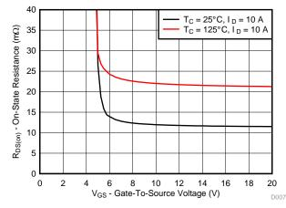
Figure 12. On-State Resistance as a Function of Gate-to-Source Voltage of CSD19537Q3
