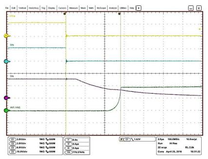
Figure 30. OFF Delay Waveforms From Logic Disable Input (Yellow) to TP9 (Blue), TP6 (Purple), and Load of the MOSFETs (Green)
