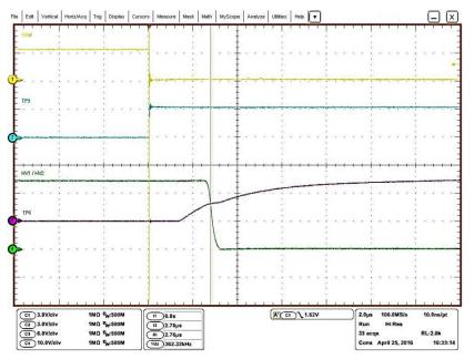
Figure 29. ON Delay Waveforms From Logic Enable Input (Yellow) to TP9 (Blue), TP6 (Purple), and Load of the MOSFETs (Green)
