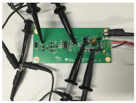
Figure 25. Probe Connections for Signal Chain Waveforms
