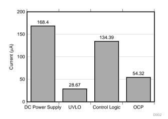
Figure 27. Steady-State Current Consumption During OFF Time
