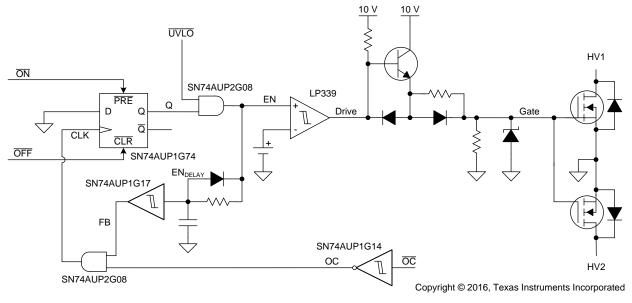
Figure 19. Control Logic and Gate Driver Schematic
