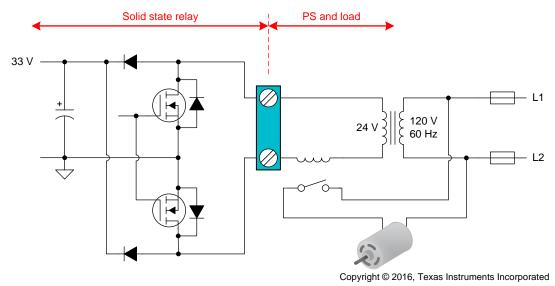
Figure 10. Power Supply of SSR in HVAC System
