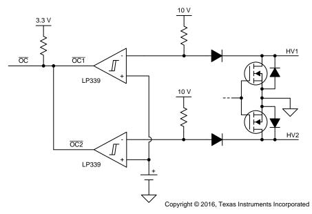
Figure 17. Simplified Schematic of OCP
