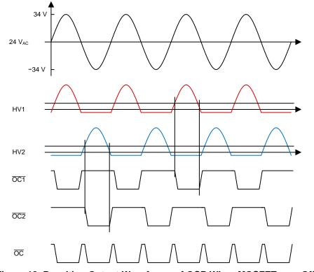
Figure 18. Resulting Output Waveforms of OCP When MOSFETs are Off
