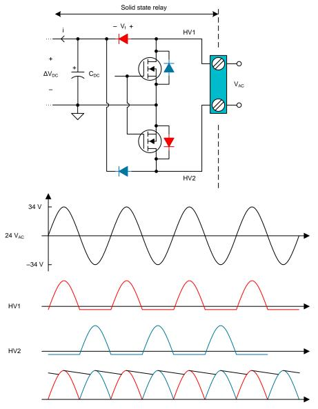
Figure 11. Full-Wave Rectification Circuitry and Waveforms
