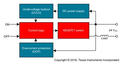
Figure 1. TIDA-00377 SSR With MOSFETs Block Diagram
