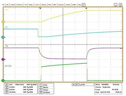
Figure 28. Charging Time of DC Supply Capacitor (Yellow) in Reference to TP1 (Blue), TP6 (Purple), and HV1/HV2 (Green)
