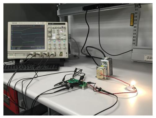
Figure 24. Test Setup of TIDA-00337 EVM, Light Bulb, and Transformer
