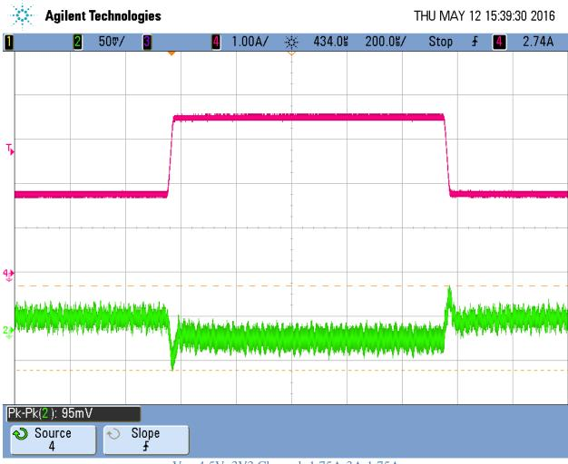
V<sub>IN</sub>=4.5V, 3V3 Channel: 1.75A-3A-1.75A
