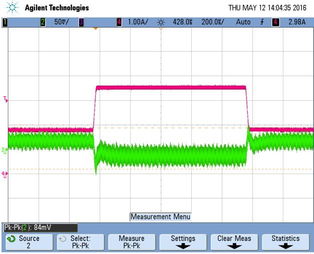
V<sub>IN</sub>=9V, 3V3 Channel: 1.75A-3A-1.75A
