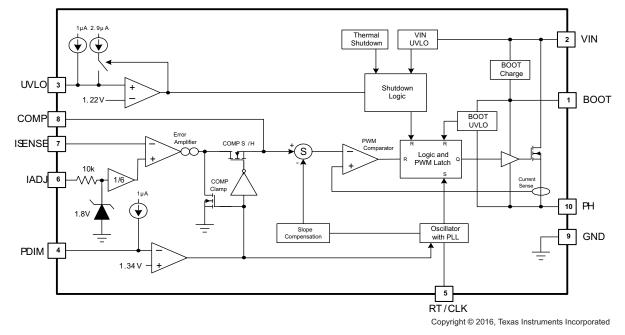
Figure 3. TPS92513 Functional Block Diagram
