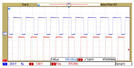
Figure 32. PH Pin Voltage—RT/CLK Pin PWM Input at 1000 kHz
