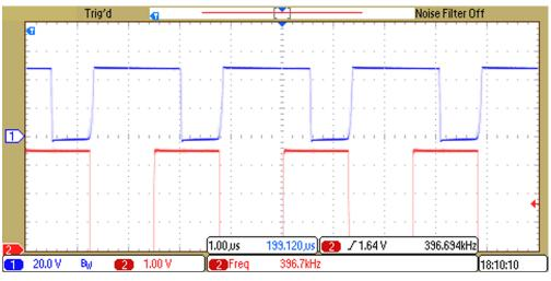
Figure 31. PH Pin Voltage—RT/CLK Pin PWM Input at 400 kHz
