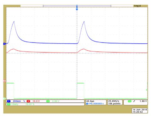
Figure 21. LED Current, LED Voltage, and PDIM Input Waveforms at 10% Duty Cycle
