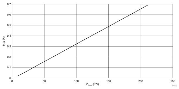
Figure 11. LED Driver Current Output Linearity With VIADJ
