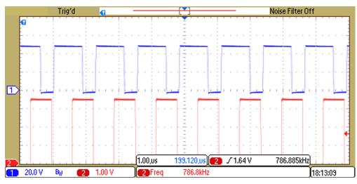
Figure 28. PH Pin Voltage—RT/CLK Pin PWM Input at 800 kHz
