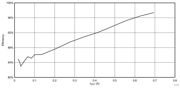
Figure 13. Individual TPS92513 Driver Efficiency With 1-kHz PWM Dimming
