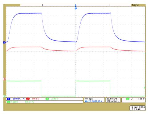
Figure 20. LED Current, LED Voltage, and PDIM Input Waveforms at 50% Duty Cycle
