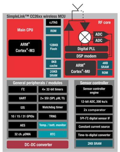
Figure 5. CC2650 Block Diagram
