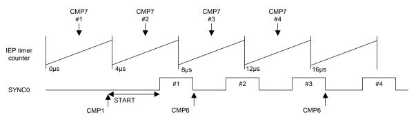
Figure 11. SYNC0 Pulse Generation With Overlap Pulse Generated in Previous Cycle
