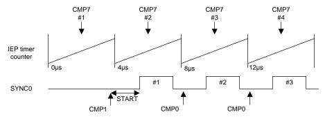
Figure 10. SYNC0 Pulse Generation With No-Overlap Pulse Generated in Previous Cycle
