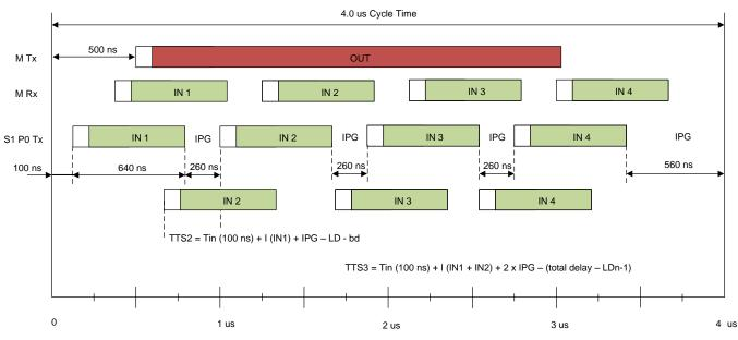
Figure 3. 4-µs Control Cycle Time of SORTE Protocol
