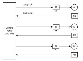
Figure 1. Traditional CNC Wiring Between Control Unit and Motor Units
