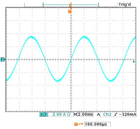
Figure 13. Stepper Motor Current for 1/256 Microstepping
