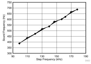
Figure 7. Sound Curve of Stepper Motors With Metal Plate
