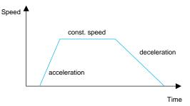
Figure 4. Speed Profile for Stepper Motor
