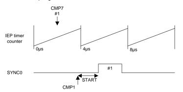
Figure 9. SYNC0 Generation With No Pulse Generated in Previous Cycle Time
