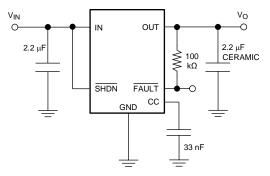
Figure 6. LP3982 Typical Application (Fixed V<sub>out</sub> Version)
