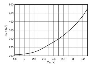
Figure 1. MSP430 Current Consumption Based on V<sub>cc</sub>
