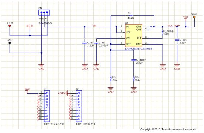
Figure 10. TIDA-01172 Schematic
