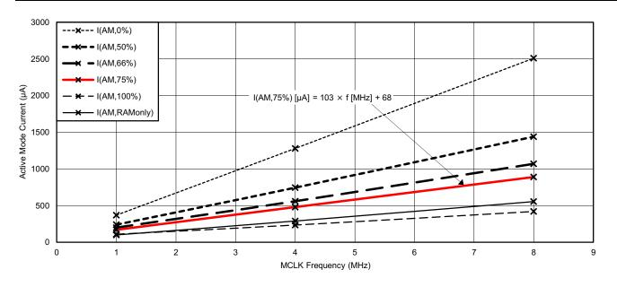
Figure 3. Typical Characteristics - Active Mode Supply Currents for MSP430
