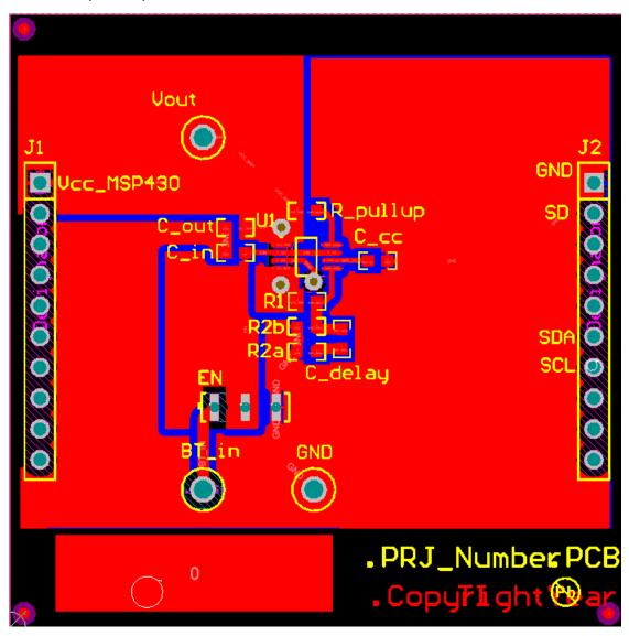
Figure 11. PCB Layout Guidelines
