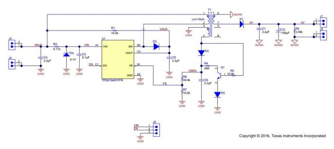
Figure 1. Reference Design Schematic
