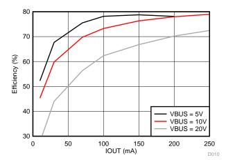
Figure 9. Efficiency of Secondary-Side Regulation Solution
