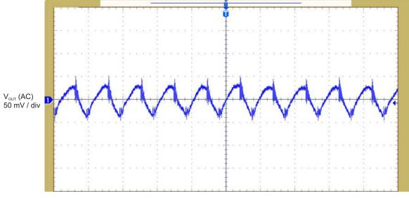
Figure 5. V<sub>OUT</sub> Ripple at V<sub>IN</sub> = 10 V and I<sub>OUT</sub> = 250 mA
