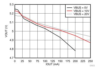
Figure 2. Load Regulation of Primary-Side Regulation Solution (V<sub>out</sub> = 5 V)
