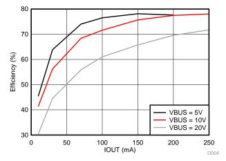
Figure 3. Efficiency of Primary-Side Regulation Solution
