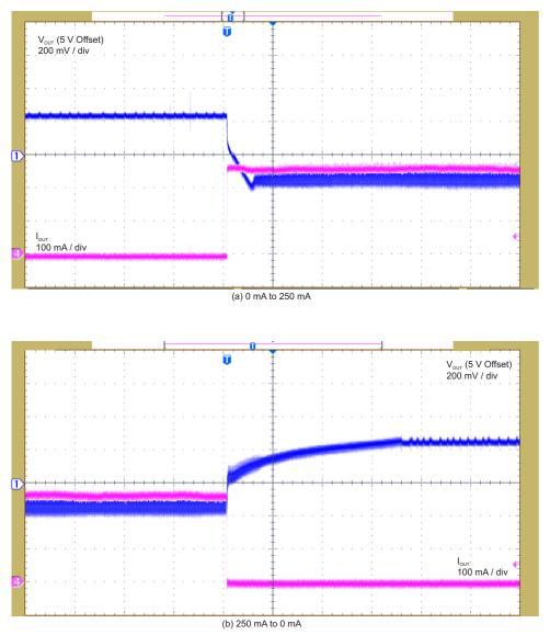
Figure 6. V<sub>out</sub> Ripple at Load Transient
