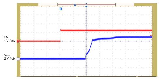
Figure 10 shows the start-up waveform of the secondary-side regulation solution at  $I_{OUT}$ = 10 mA and  $V_{BUS}$ = 10 V.
