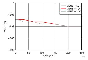
Figure 8. Load Regulation of Secondary-Side Regulation Solution
