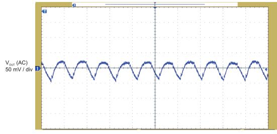
Figure 11.  $V_{\text{out}}$  Ripple of Secondary-Side Regulation Solution
