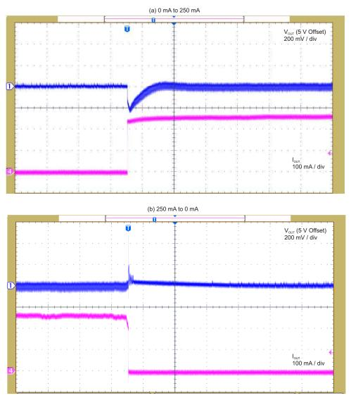
Figure 12. Load Transient of Secondary-Side Regulation Solution
