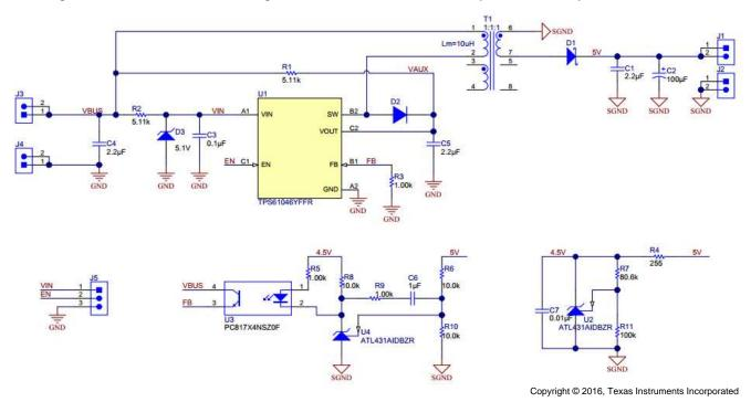
Figure 7. Secondary-Side Regulation Solution
