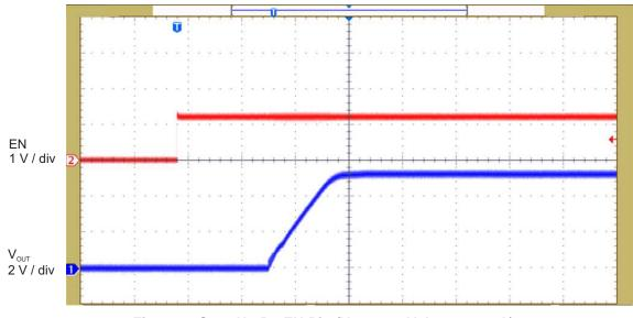
Figure 4. Start Up By EN Pin ( $V_{BUS} = 10 \text{ V}, I_{OUT} = 10 \text{ mA}$ )
