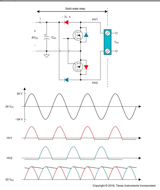
Figure 5. Full-Wave Rectification Waveforms
