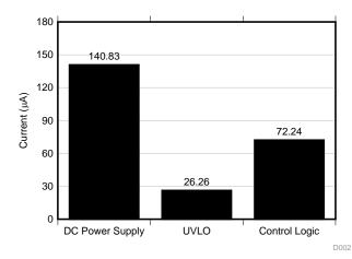
Figure 18. Measured Steady-State Current Consumption During OFF Time
