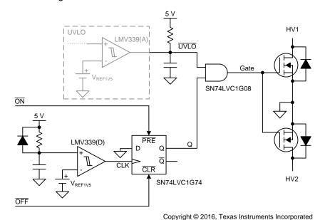
Figure 12. Control Logic and Gate Driver Schematic
