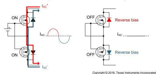
Figure 3. Functionality of MOSFETs for (a) ON and (b) OFF Times
