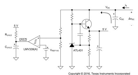
Figure 8. DC Power Supply and UVLO Circuit
