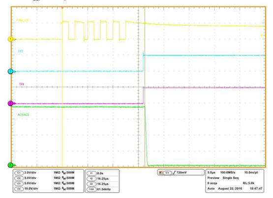
Figure 20. ON Delay Waveforms From PWM ON Input (Yellow) to TP3 (Blue), TP4 (Purple), and  $V_{\rm DS}$  of MOSFETs (Green)
