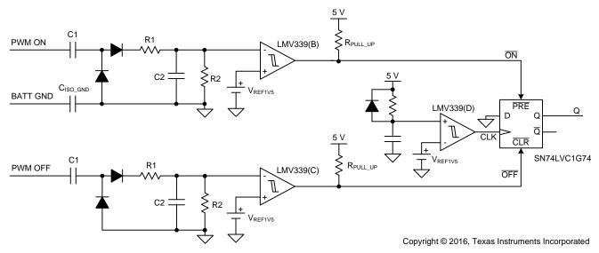
Figure 10. Capacitive Isolation Network With Logic Control
