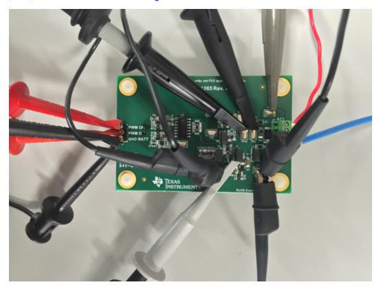
Figure 16. Probe Connections for Signal Chain Waveforms
