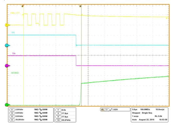
Figure 21. OFF Delay Waveforms From PWM OFF Input (Yellow) to TP3 (Blue), TP4 (Purple), and V<sub>DS</sub> of MOSFETs (Green)
