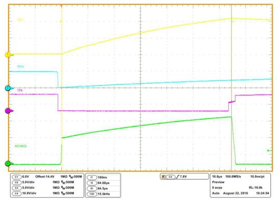
Figure 19. Charging Time of DC Supply Capacitor (Yellow) in Reference to TP10 (Blue), TP4 (Purple), and AC1/AC2 (Green)
