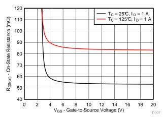
Figure 6. On-State Resistance as Function of Gate-to-Source Voltage of CSD18541F5
