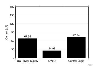
Figure 17. Measured Steady-State Current Consumption During ON Time
