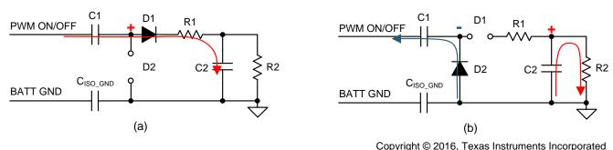
Figure 11. Mode of Isolation Network During (a) V<sub>HIGH</sub> and (b) V<sub>LOW</sub> of PWM Input Signal
