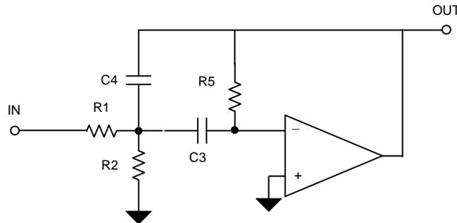
Figure 2. Multiple Feedback Band-Pass Filter (Single-Ended)
