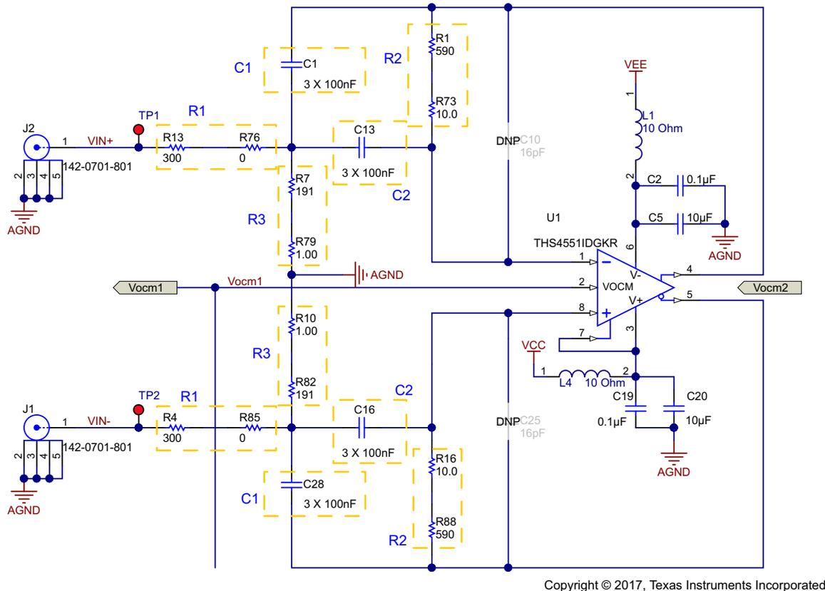
Figure 5. Differential Band-Pass Filter
