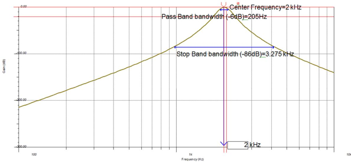
Figure 8. TINA Simulation—Frequency Response
