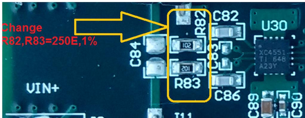
**Figure 15. TIDA-01035 Resistor Change Location**
