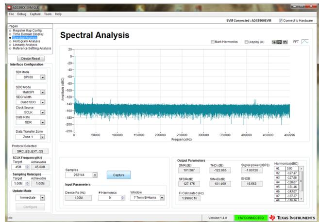
Figure 17. Spectrum With TIDA-01036 Filter
